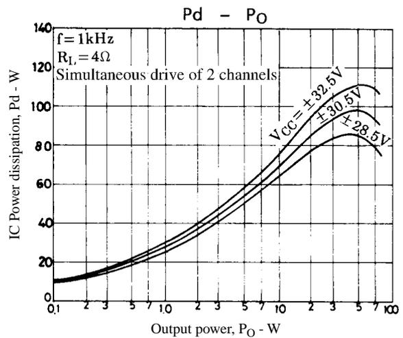
Figure 2. STK4182II Pd - P<sub>O</sub> (R<sub>L</sub> = 4Ω)
