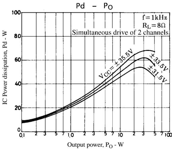
Figure 1. STK4182II Pd - P<sub>O</sub> (R<sub>L</sub> = 8Ω)
