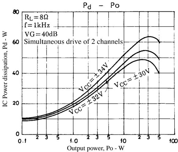
Figure 1. STK4172II Pd - Po ( $R_L = 8\Omega$ )
