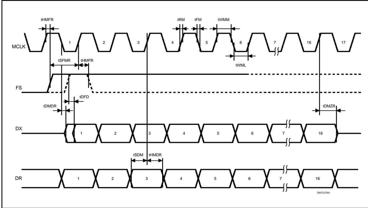
(\*) In the case of companded code the timing is applied to 8 bits instead of 16 bits.
