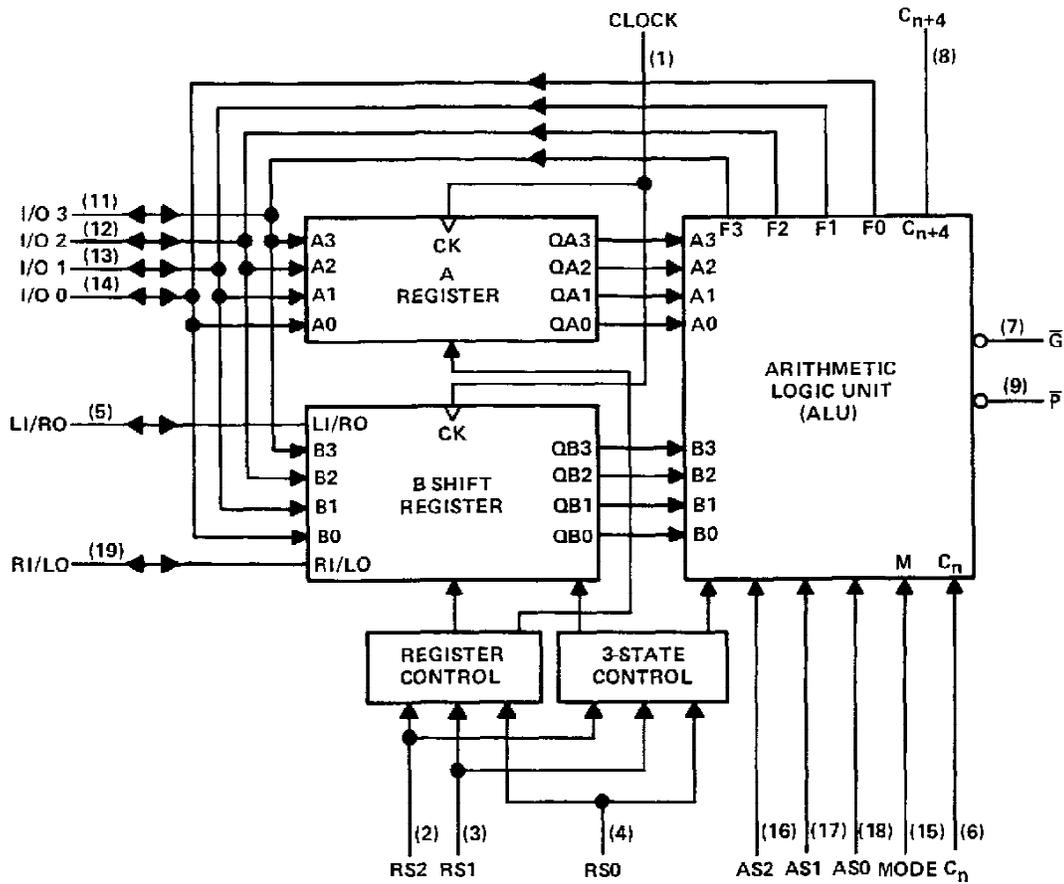
schematics of inputs and outputs
