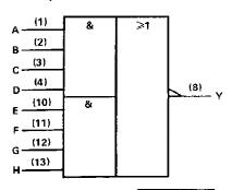
positive logic:  $Y = \overline{ABCD + EFGH}$
