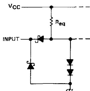
Data select and strobe  $R_{req} = 20 \text{ k}\Omega \text{ NOM}$
