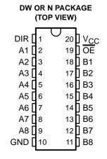
(DIR) input. The output-enable (OE) input can be used to disable the device so that the buses are effectively isolated. The SN74ALS1640A features inverting logic, while the SN74ALS1645A features noninverting logic.
