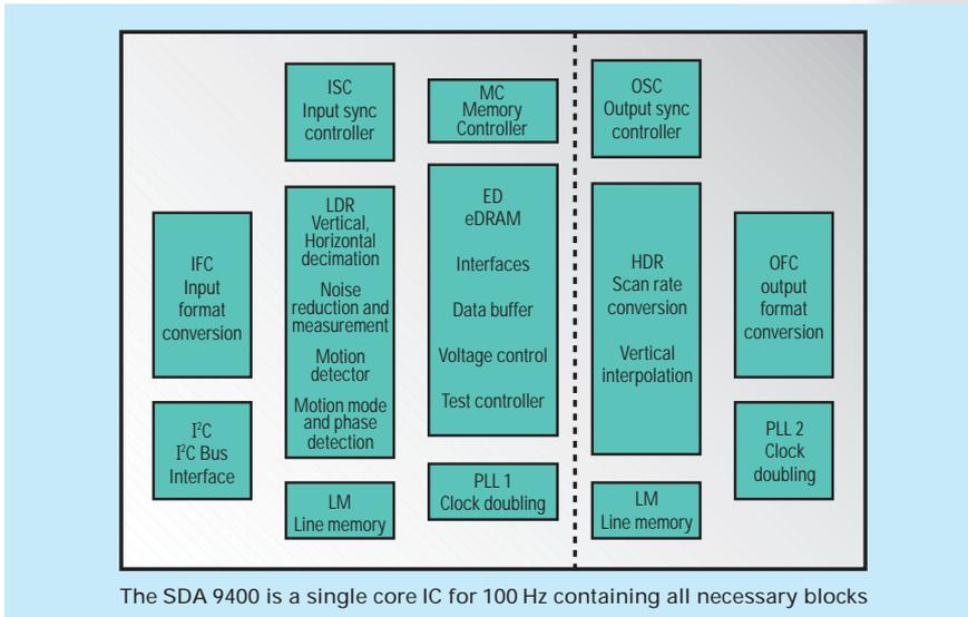
The SDA 9400 contains all necessary functional blocks on a single chip:
