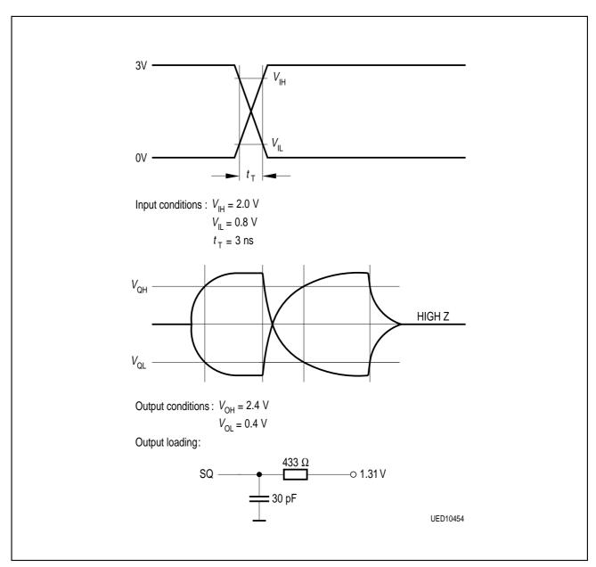
Diagram 1 AC-Timing Measuring Conditions
