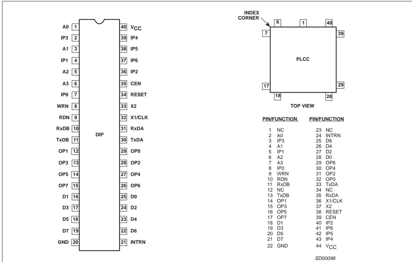
Figure 1. Pin Configurations
