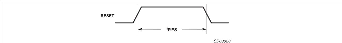
Figure 3. Reset Timing
