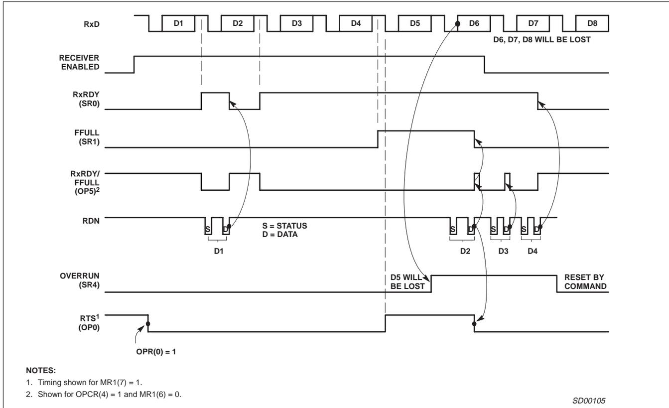
Figure 11. Receiver Timing
