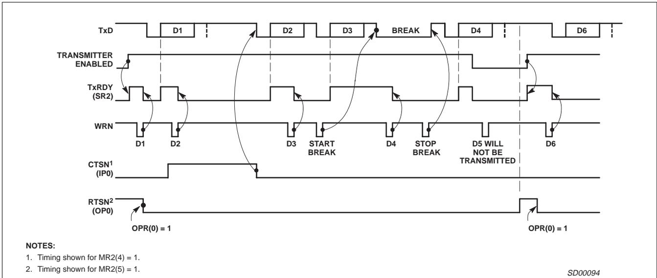
Figure 10. Transmitter Timing
