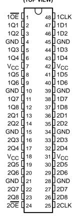
A buffered output-enable  $(\overline{OE})$  input can be used to place the eight outputs in either a normal logic state (high or low logic levels) or a high-impedance state. In the high-impedance state, the outputs neither load nor drive the bus lines significantly. The high-impedance state and the increased drive provide the capability to drive bus lines without need for interface or pullup components.
