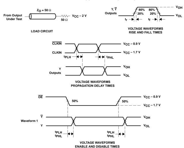
NOTES: A. All input pulses are supplied by generators having the following characteristics: PRR  $\leq$  45 MHz,  $Z_O = 50 \Omega$ ,  $t_r \leq 1$  ns.
