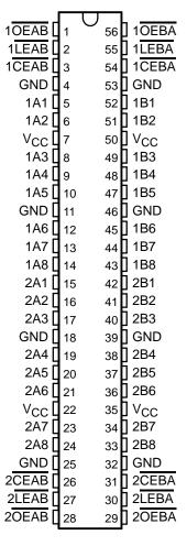
The A-to-B enable (CEAB) input must be low to enter data from A or to output data from B. If CEAB is low and LEAB is low, the A-to-B latches are transparent; a subsequent low-to-high transition of LEAB puts the A latches in the storage mode. With CEAB and OEAB both low, the 3-state B outputs are active and reflect the data present at the output of the A latches. Data flow from B to A is similar, but requires using the CEBA, LEBA, and OEBA inputs.
