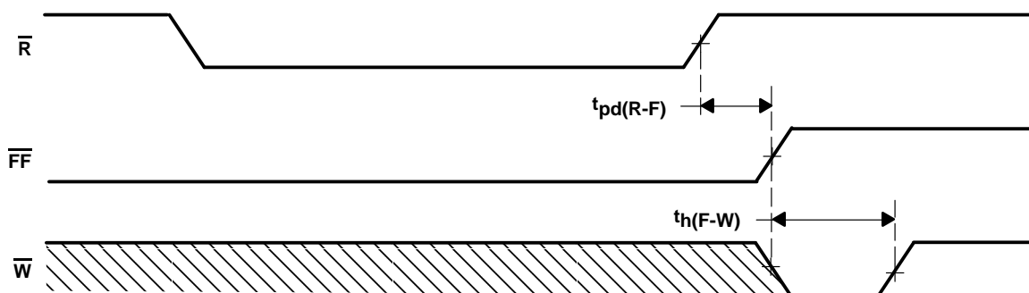
Figure 12. Minimum Timing for a Full-Flag Coincident-Write Pulse
