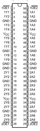
The 74ACT16825 is packaged in TI's shrink small-outline package, which provides twice the I/O pin count and functionality of standard small-outline packages in the same printed-circuit-board area.
