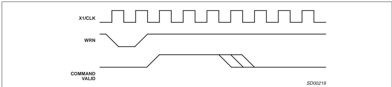
Figure 17. Command Timing
