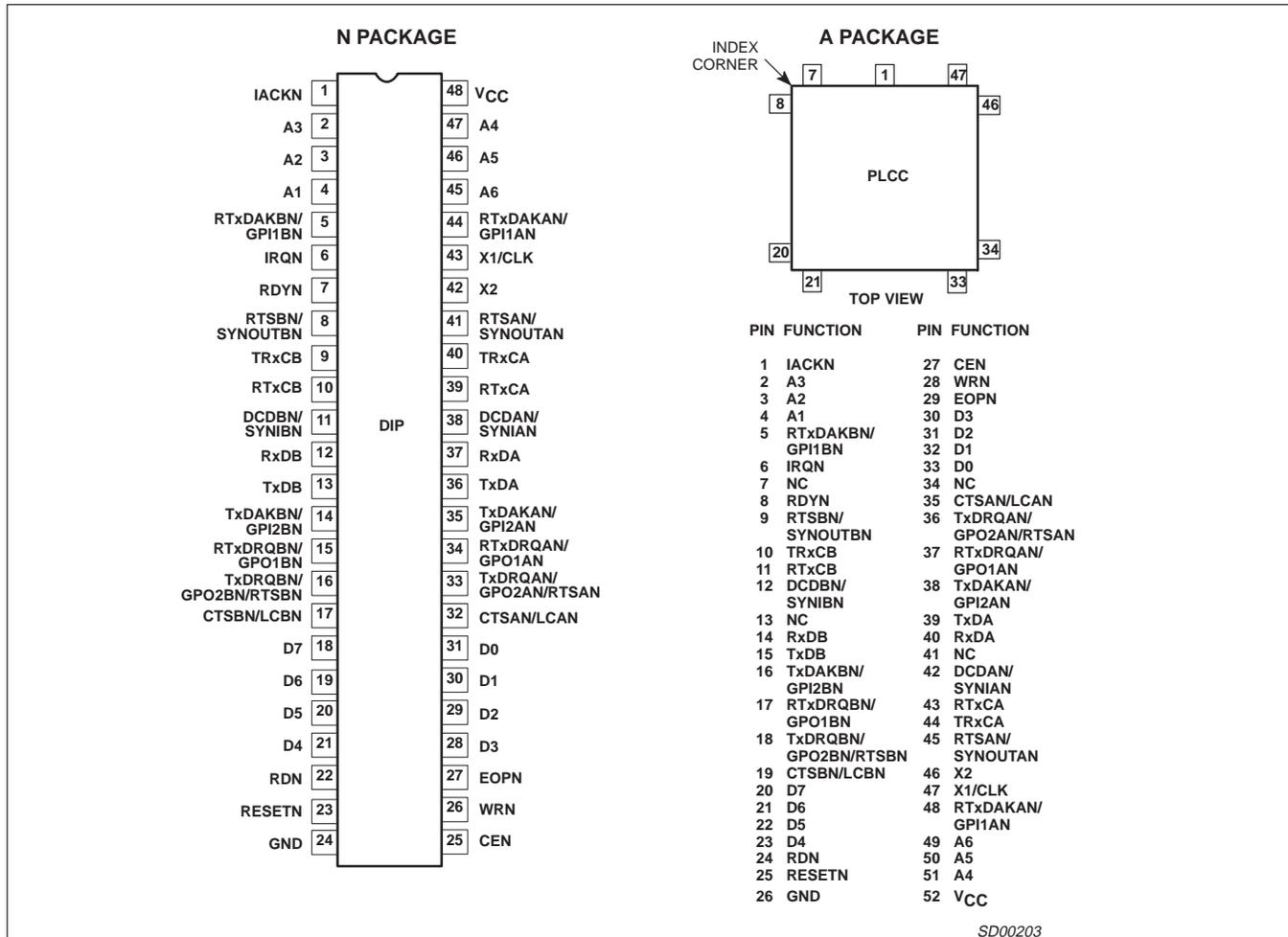
Figure 1. Pin Configurations
