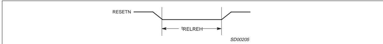
Figure 3. Reset Timing
