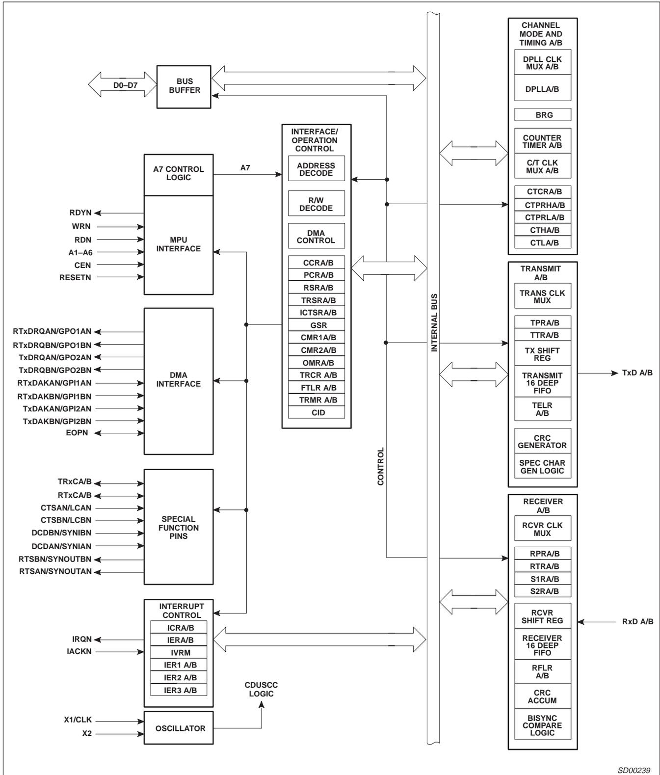
Figure 2. Block Diagram
