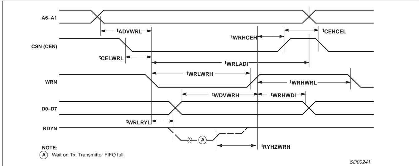
Figure 5. Write Cycle<sup>12</sup>
