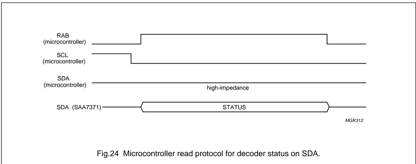
Fig.24 Microcontroller read protocol for decoder status on SDA.
