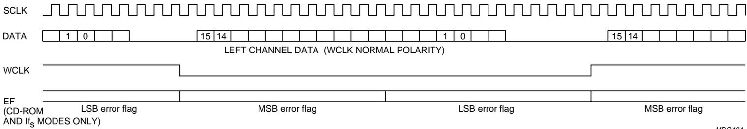
Fig.11 Philips I<sup>2</sup>S-bus data format (16-bit word length shown).
