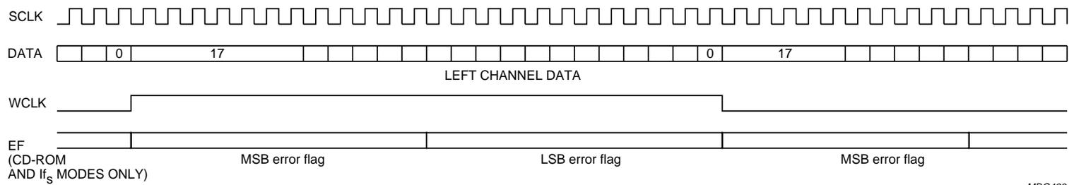
Fig.12 EIAJ data format (18-bit word length shown).
