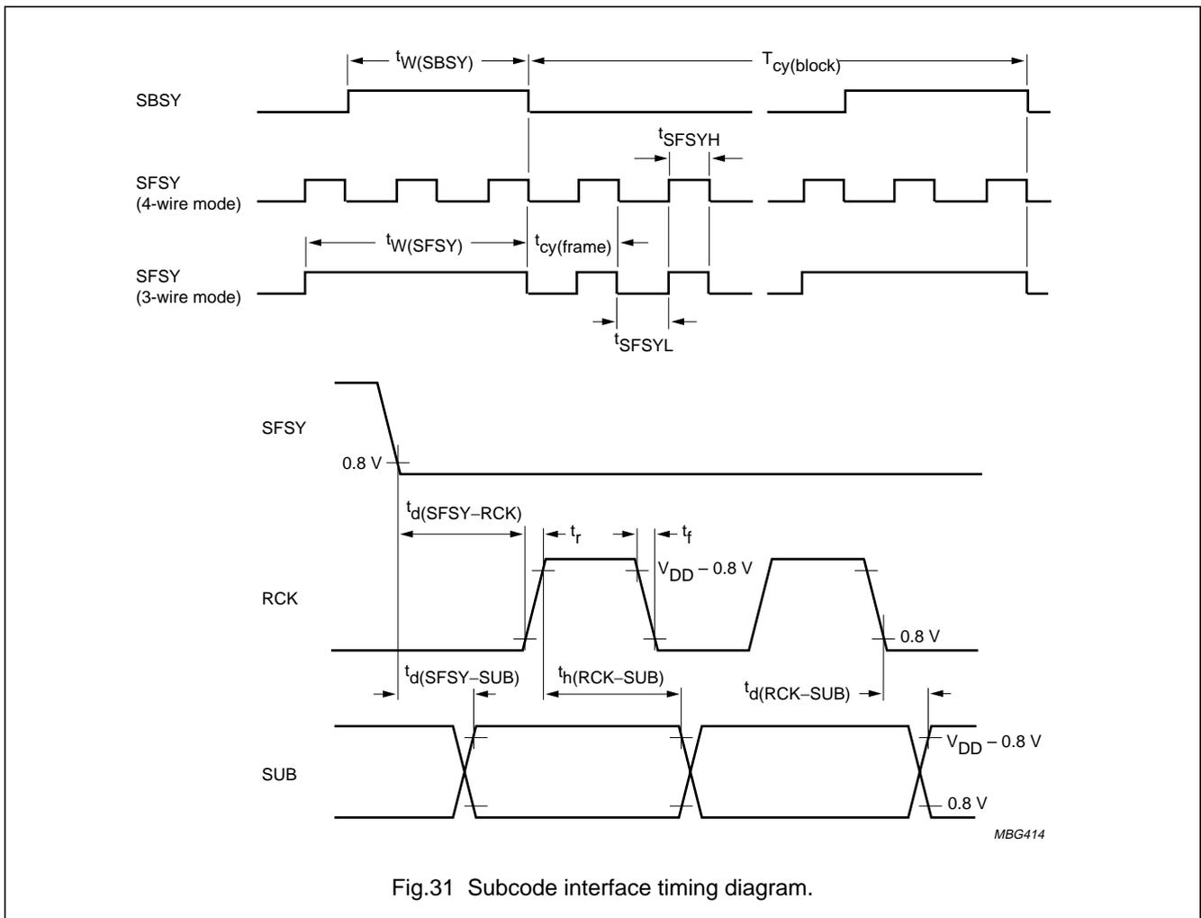
Fig.31 Subcode interface timing diagram.
