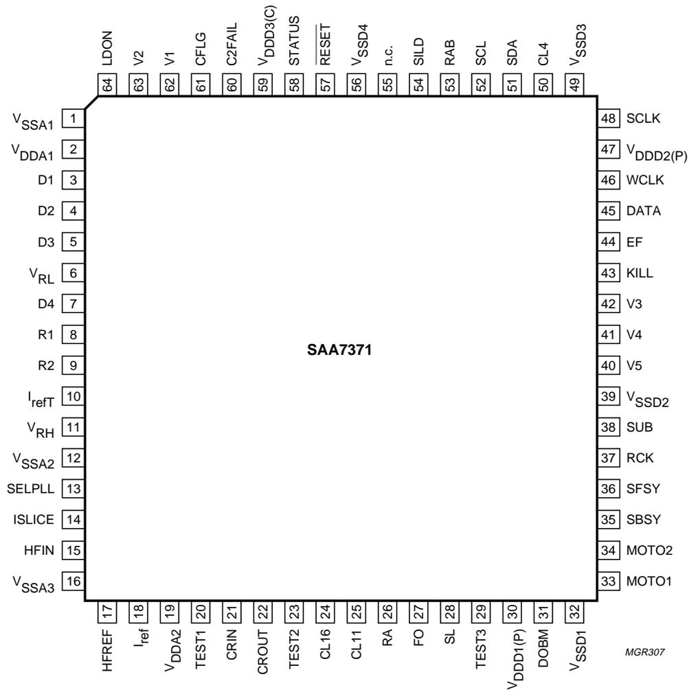
Fig.2 Pin configuration.
