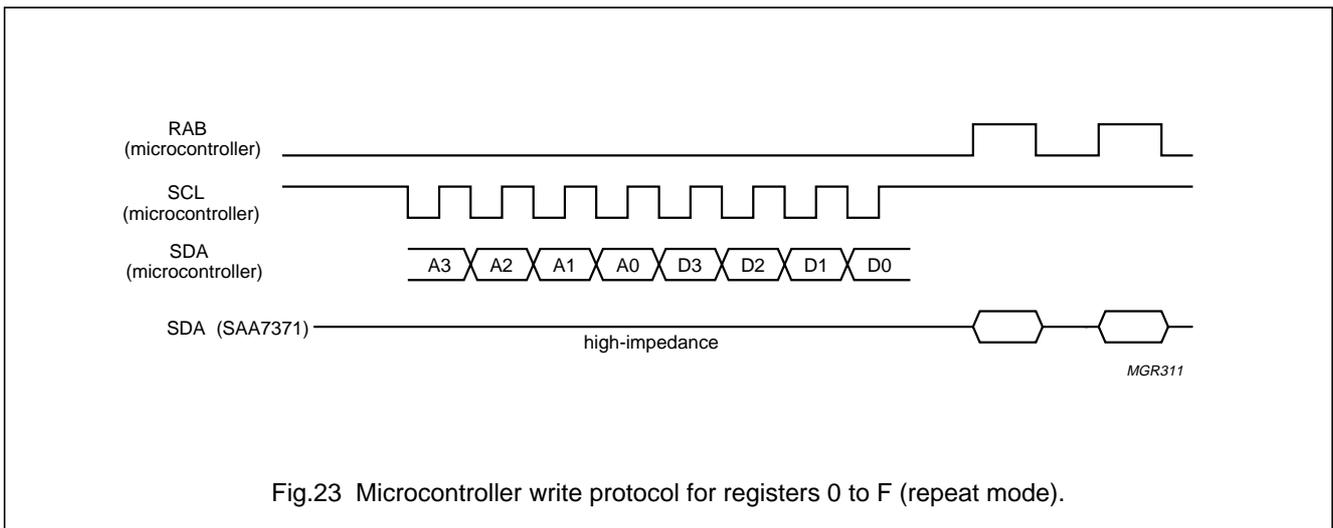
Fig.23 Microcontroller write protocol for registers 0 to F (repeat mode).
