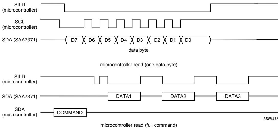
Fig.30 Microcontroller protocol for read servo commands.
