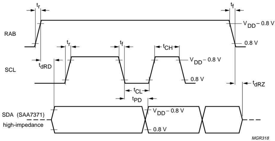
Fig.33 4-wire bus microcontroller timing; read mode (Q-channel subcode and decoder status information).
