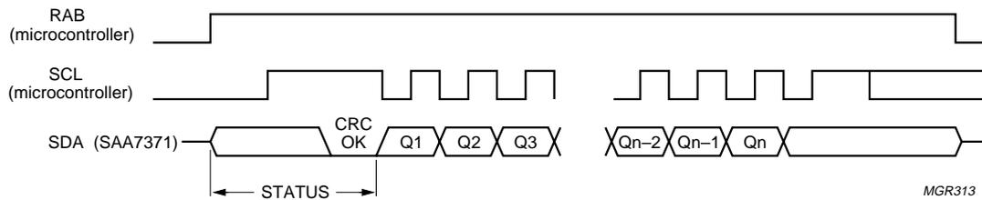
Fig.25 Microcontroller protocol for reading Q-channel subcode.
