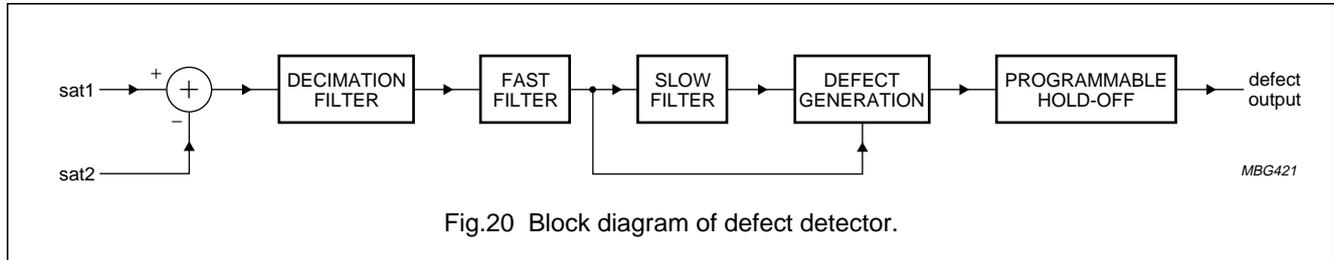
Fig.20 Block diagram of defect detector.
