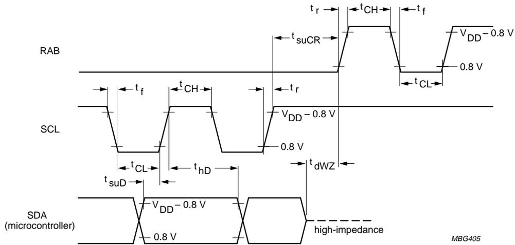
Fig.34 4-wire bus microcontroller timing; write mode (registers 0 to F).
