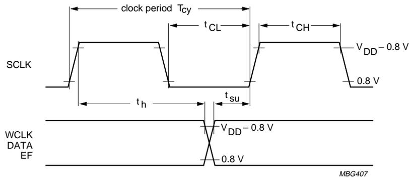
Fig.32 I<sup>2</sup>S-bus timing diagram.
