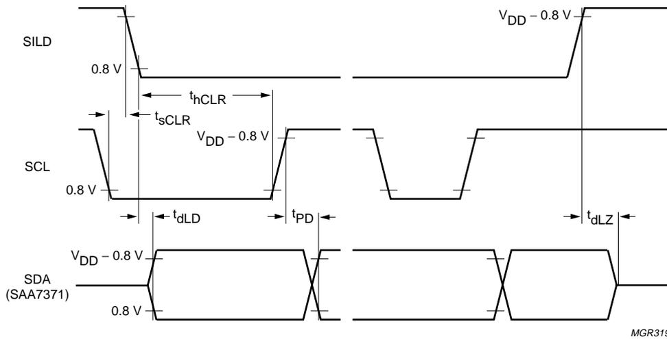
Fig.35 4-wire bus microcontroller timing; read mode (servo commands).
