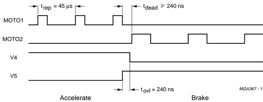
Fig.16 4-line PWM mode timing.
