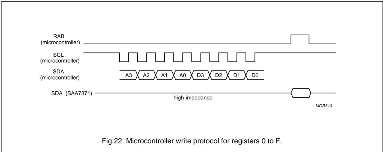
Fig.22 Microcontroller write protocol for registers 0 to F.
