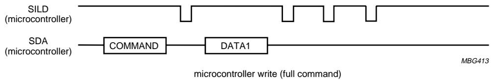
Fig.29 Microcontroller protocol for repeated data in write servo commands.
