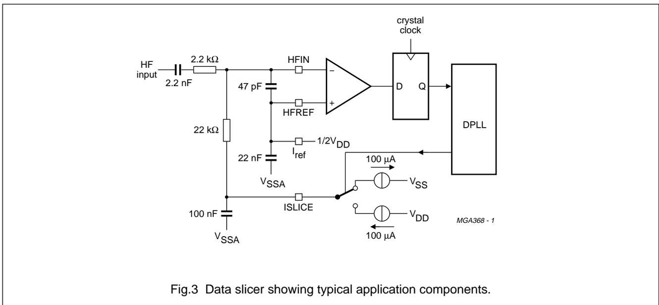
Fig.3 Data slicer showing typical application components.
