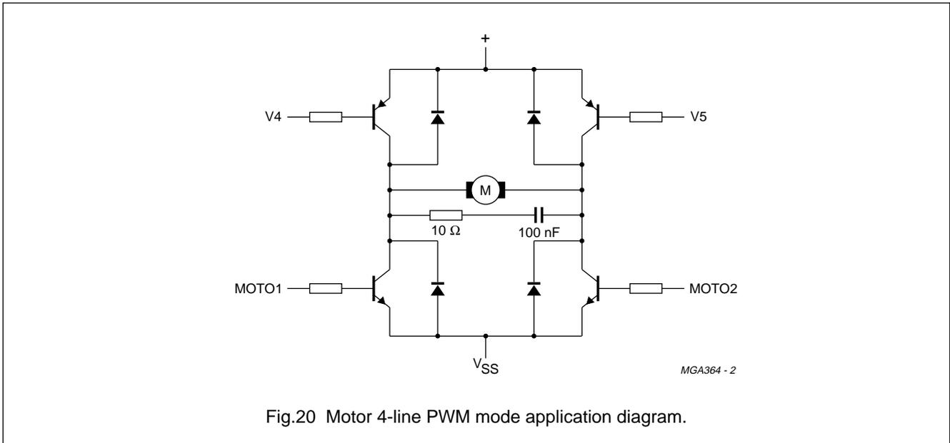
Fig.20 Motor 4-line PWM mode application diagram.
