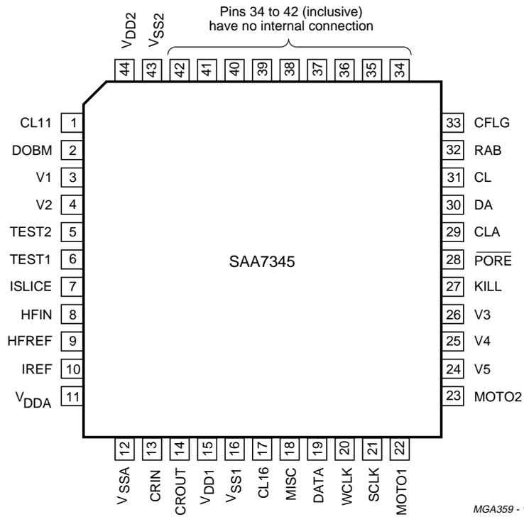
Fig.2 Pin configuration.
