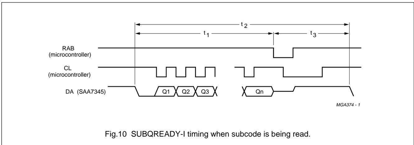
Fig.10 SUBQREADY-I timing when subcode is being read.
