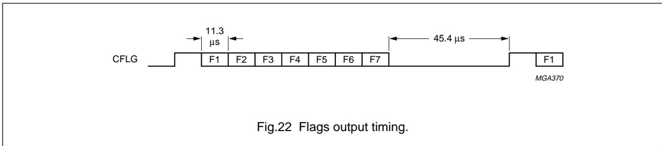
Fig.22 Flags output timing.
