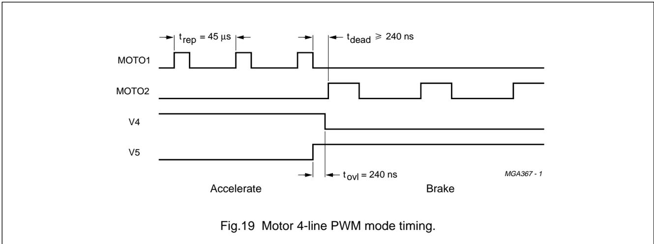
Fig.19 Motor 4-line PWM mode timing.
