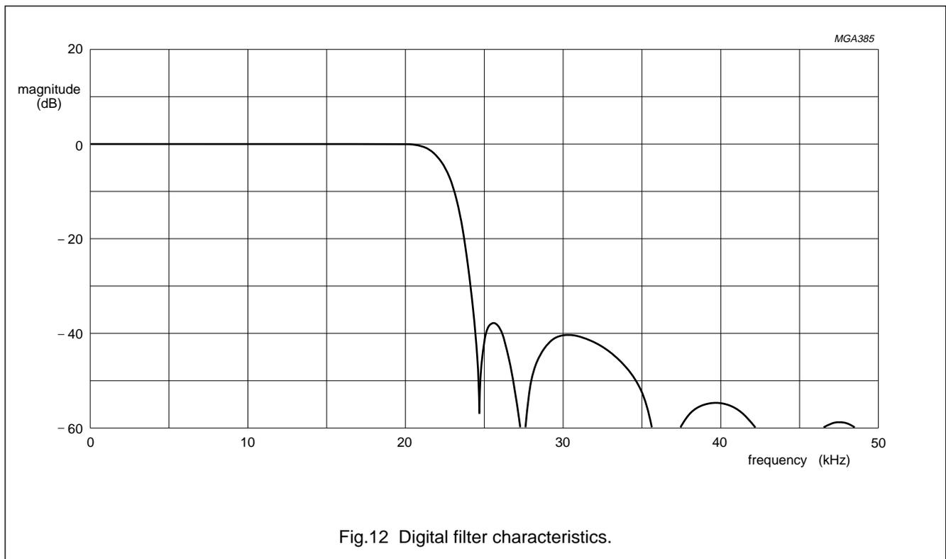
Fig.12 Digital filter characteristics.
