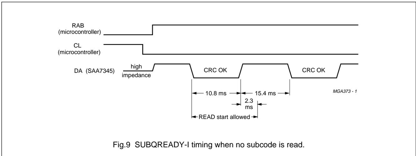
Fig.9 SUBQREADY-I timing when no subcode is read.
