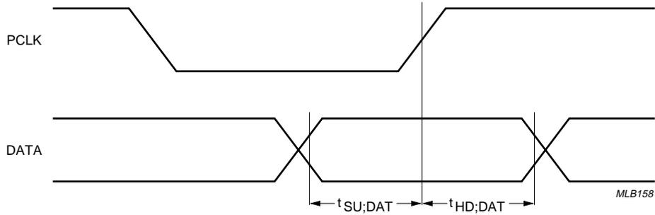
Fig.9 Data output timing.
