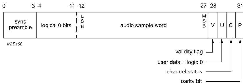
Fig.6 Sub-frame structure.
