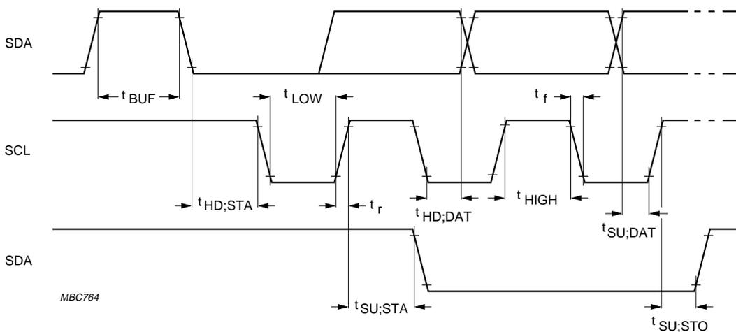
Fig.10 I<sup>2</sup>C-bus timing.
