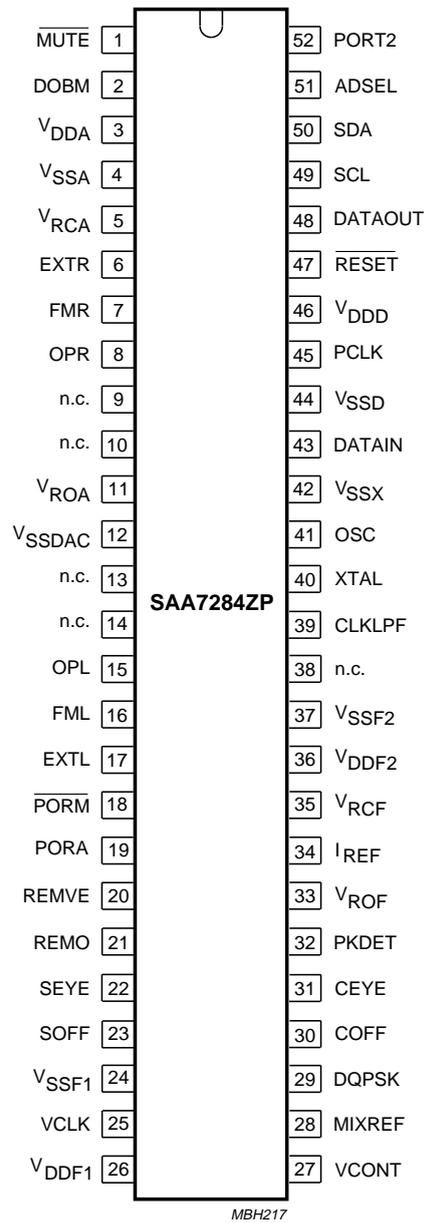
Fig.2 Pin configuration for SOT247.
