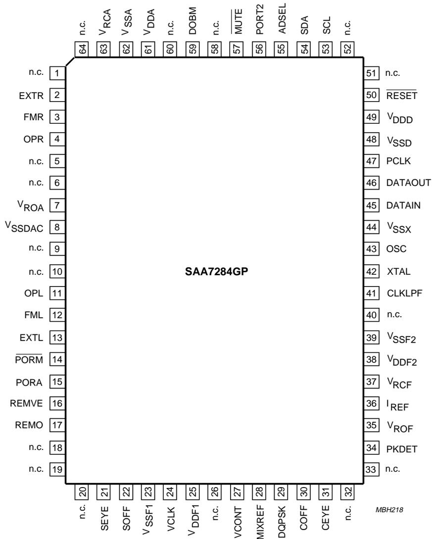
Fig.3 Pin configuration for SOT319.
