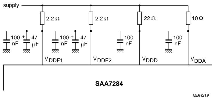
Fig.7 V<sub>DD</sub> external circuitry.
