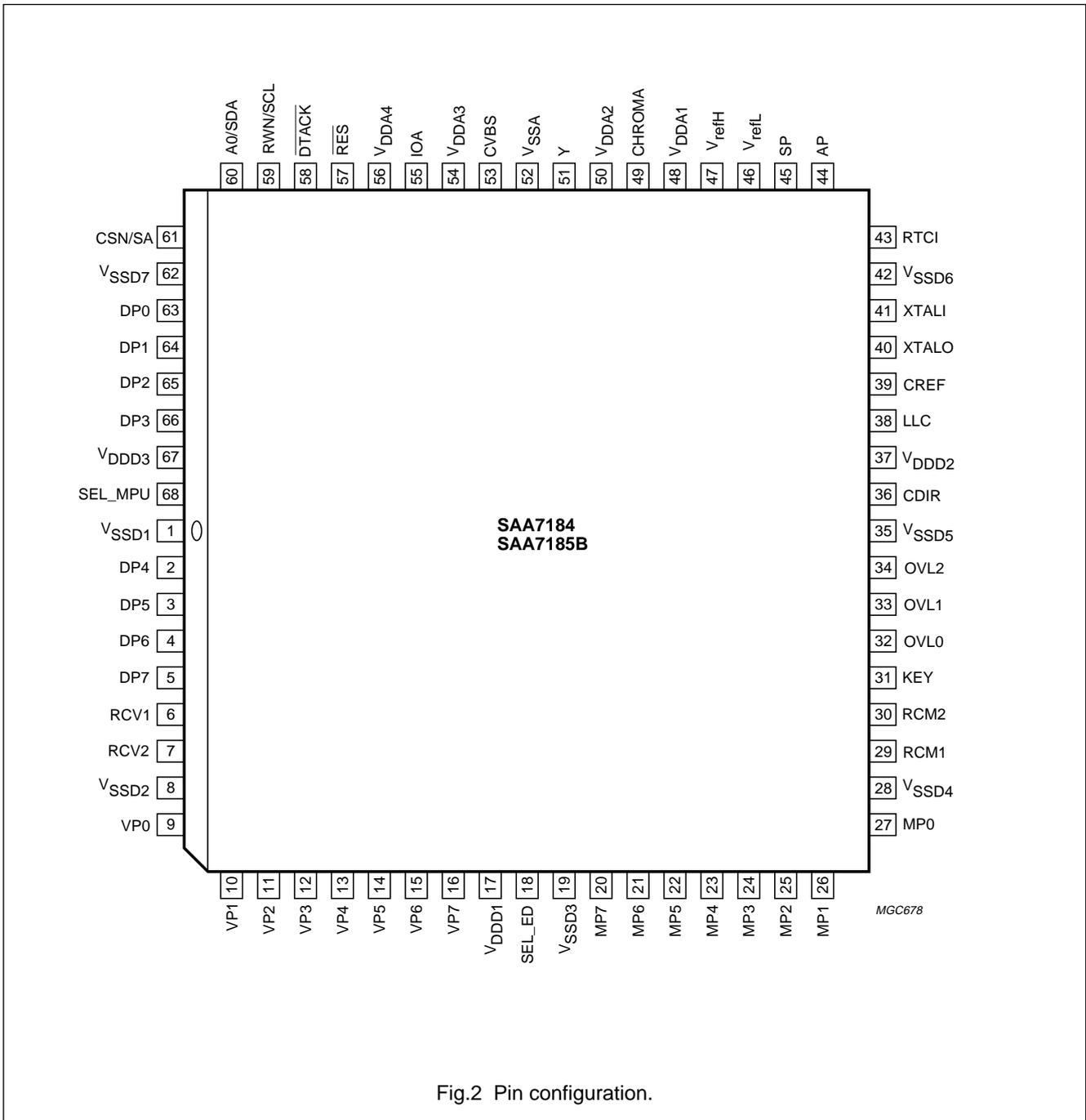
Fig.2 Pin configuration.
