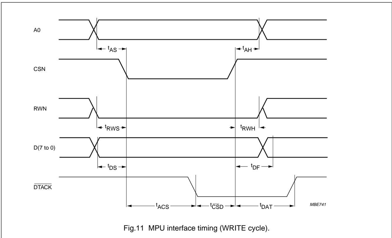
Fig.11 MPU interface timing (WRITE cycle).
