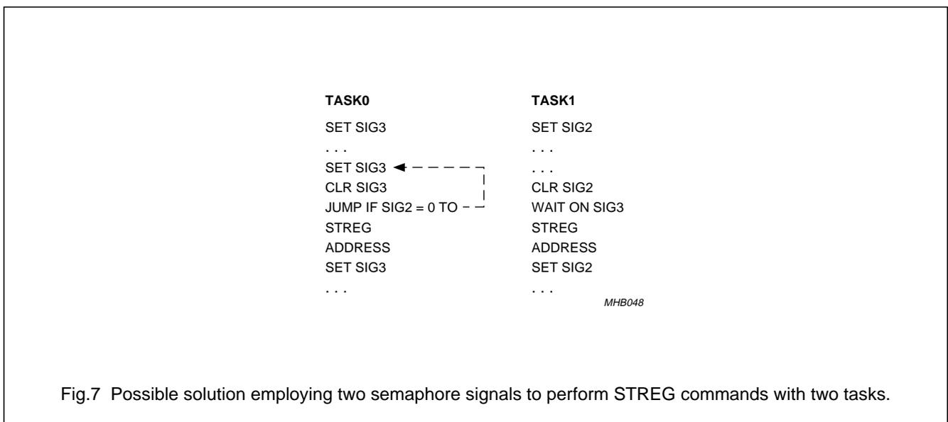
Fig.7 Possible solution employing two semaphore signals to perform STREG commands with two tasks.
