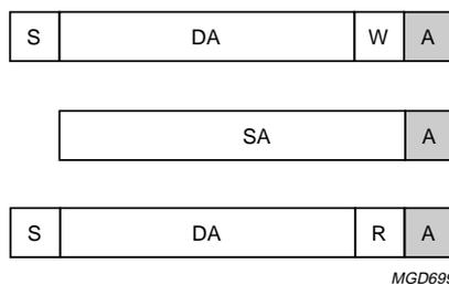
Fig.44 Address slave and write to IICTFR.
