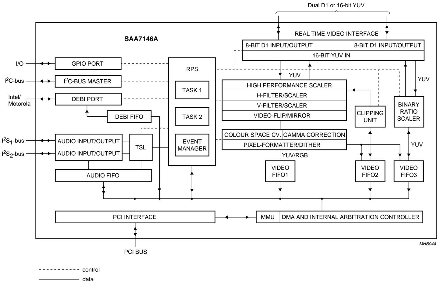
Fig.1 Block diagram.
