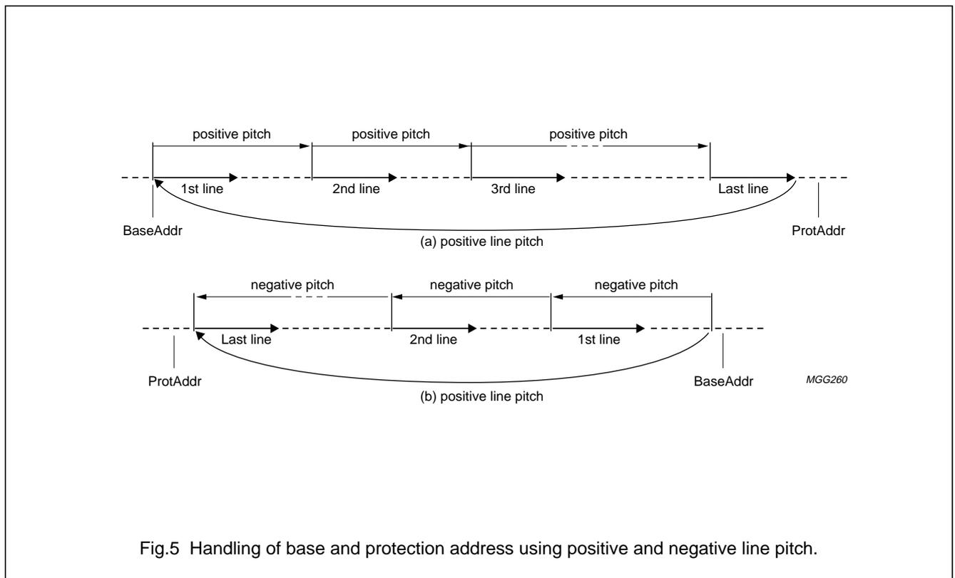
Fig.5 Handling of base and protection address using positive and negative line pitch.
