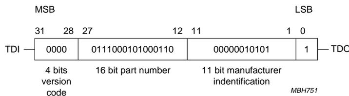
Fig.46 32 bits of identification code.
