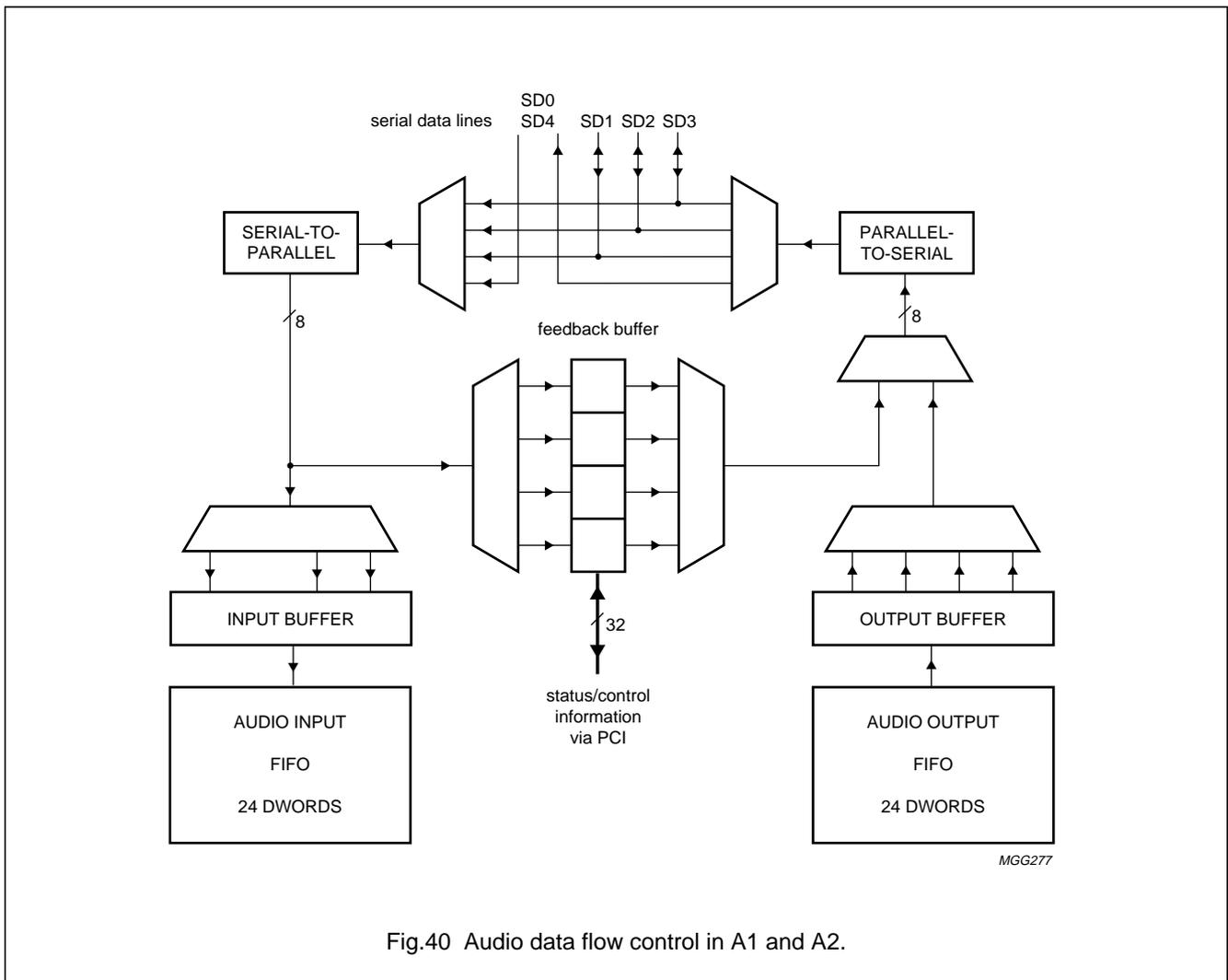
Fig.40 Audio data flow control in A1 and A2.
