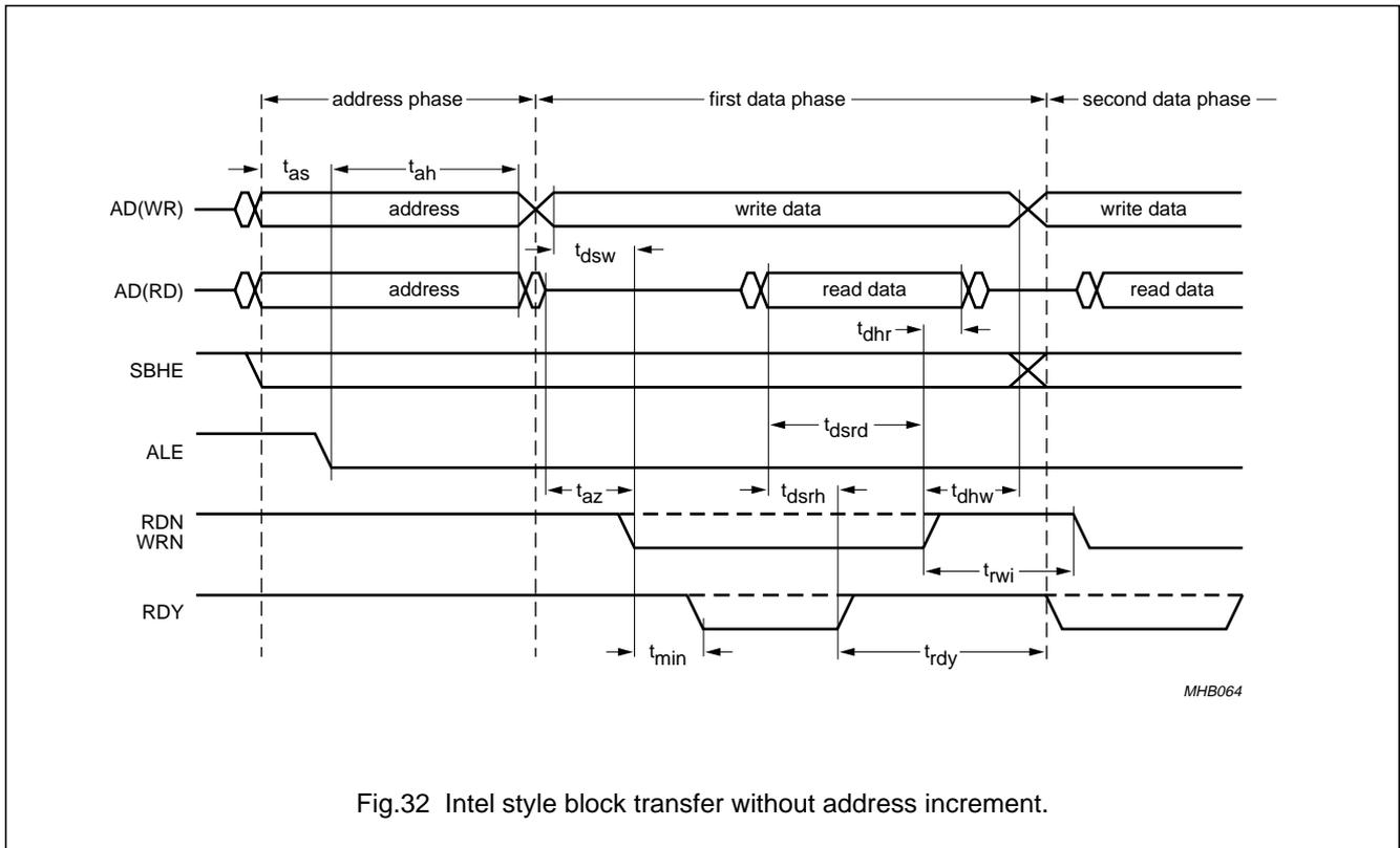
Fig.32 Intel style block transfer without address increment.
