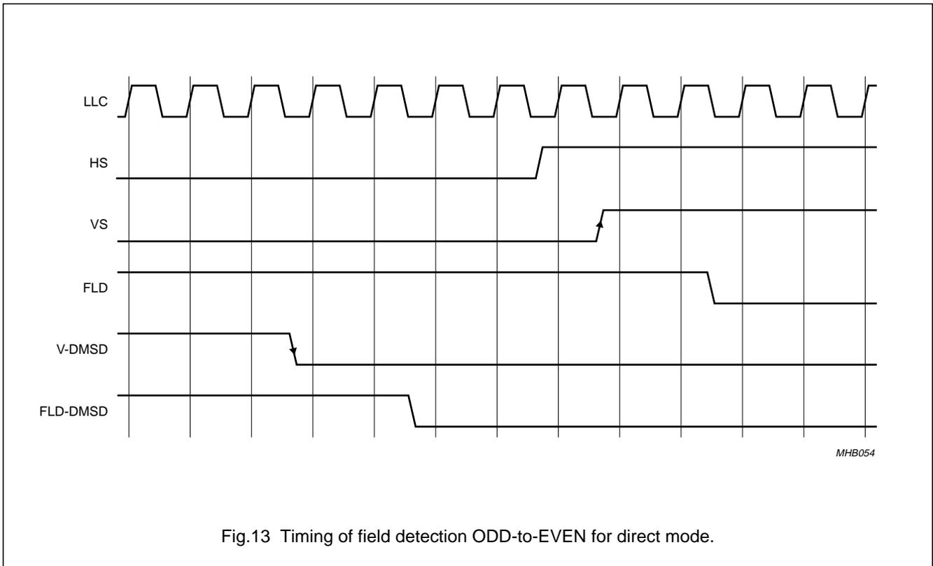
Fig.13 Timing of field detection ODD-to-EVEN for direct mode.
