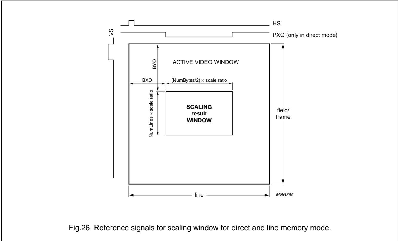
Fig.26 Reference signals for scaling window for direct and line memory mode.
