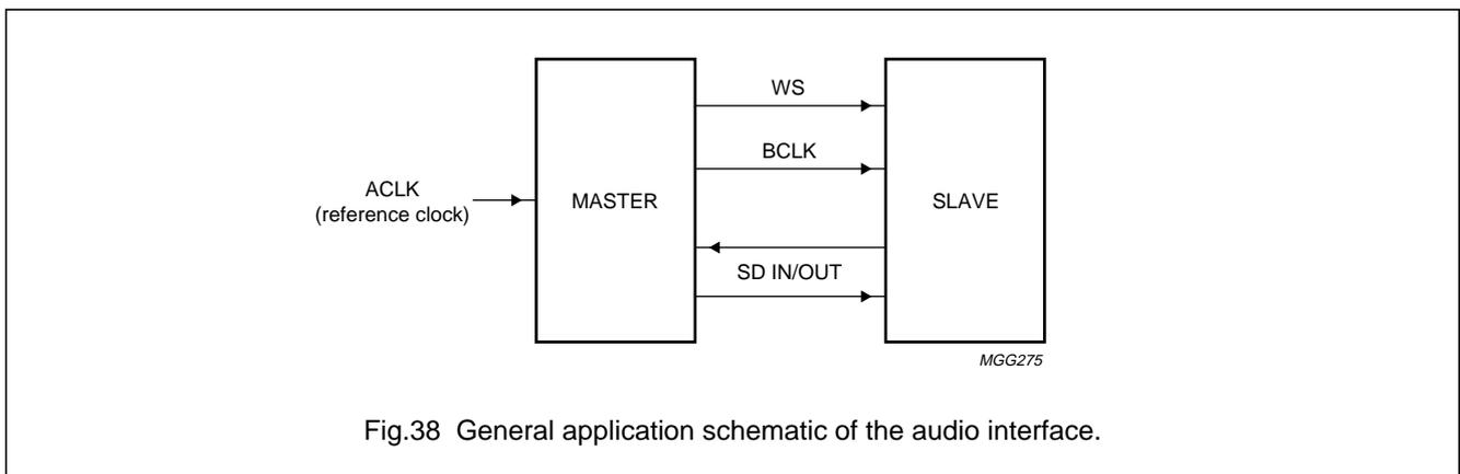
Fig.38 General application schematic of the audio interface.
