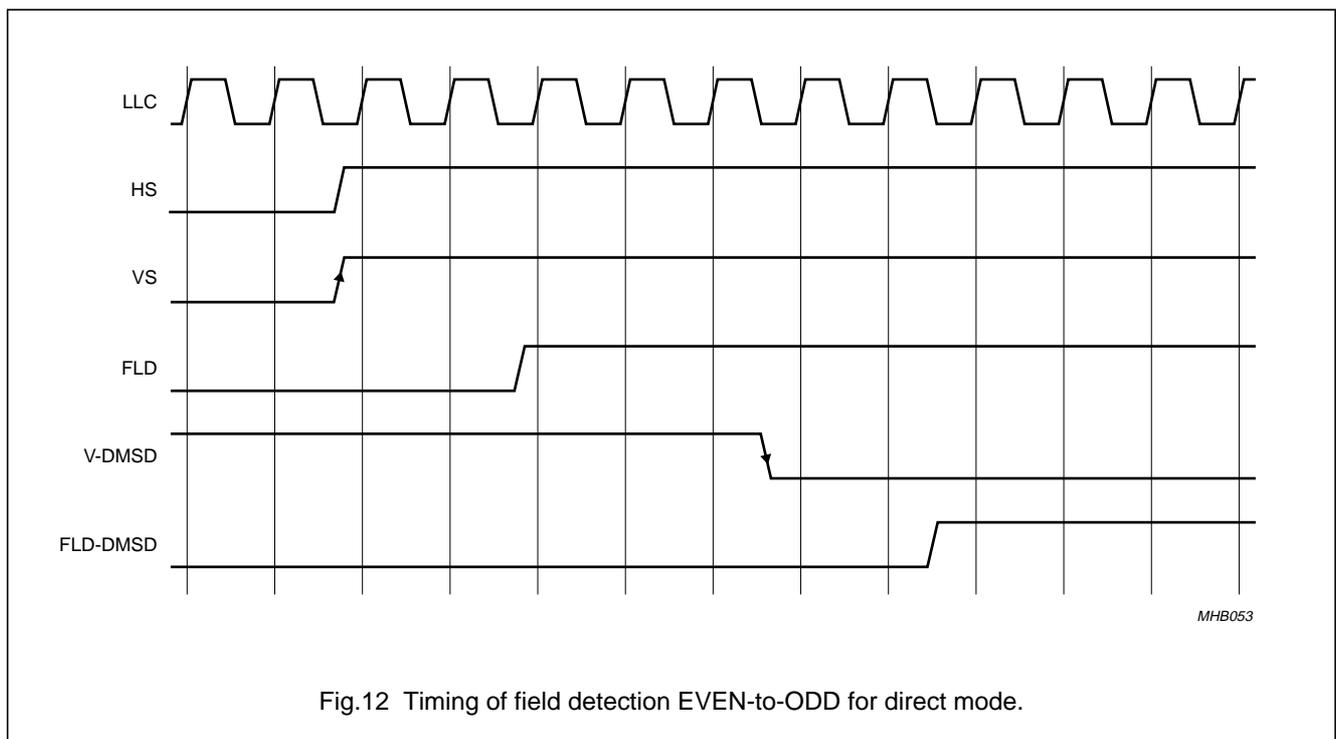
Fig.12 Timing of field detection EVEN-to-ODD for direct mode.
