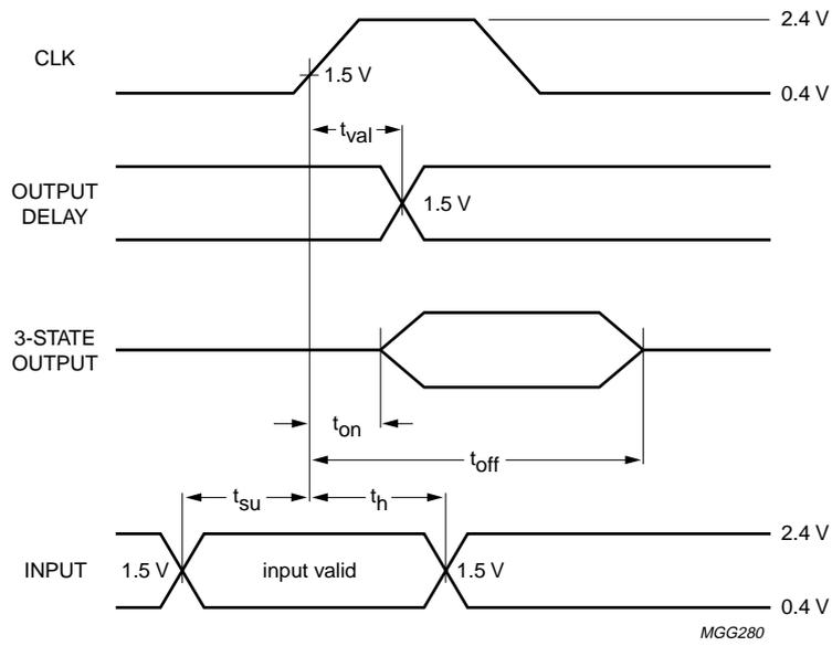
Fig.48 PCI I/O timing.
