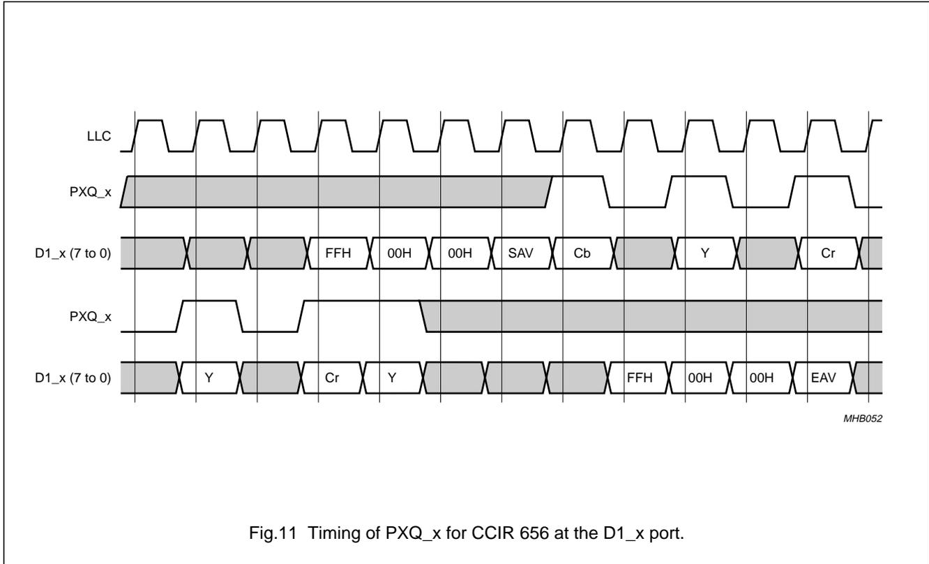
Fig.11 Timing of PXQ\_x for CCIR 656 at the D1\_x port.
