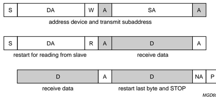
Fig.43 Protocol sequence for reading three bytes with subaddress access.
