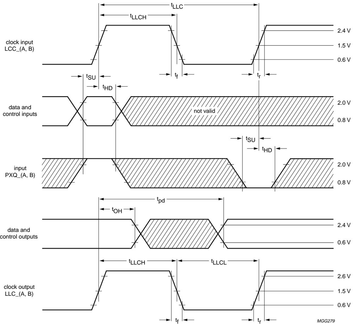
Fig.47 Clock/data timing.
