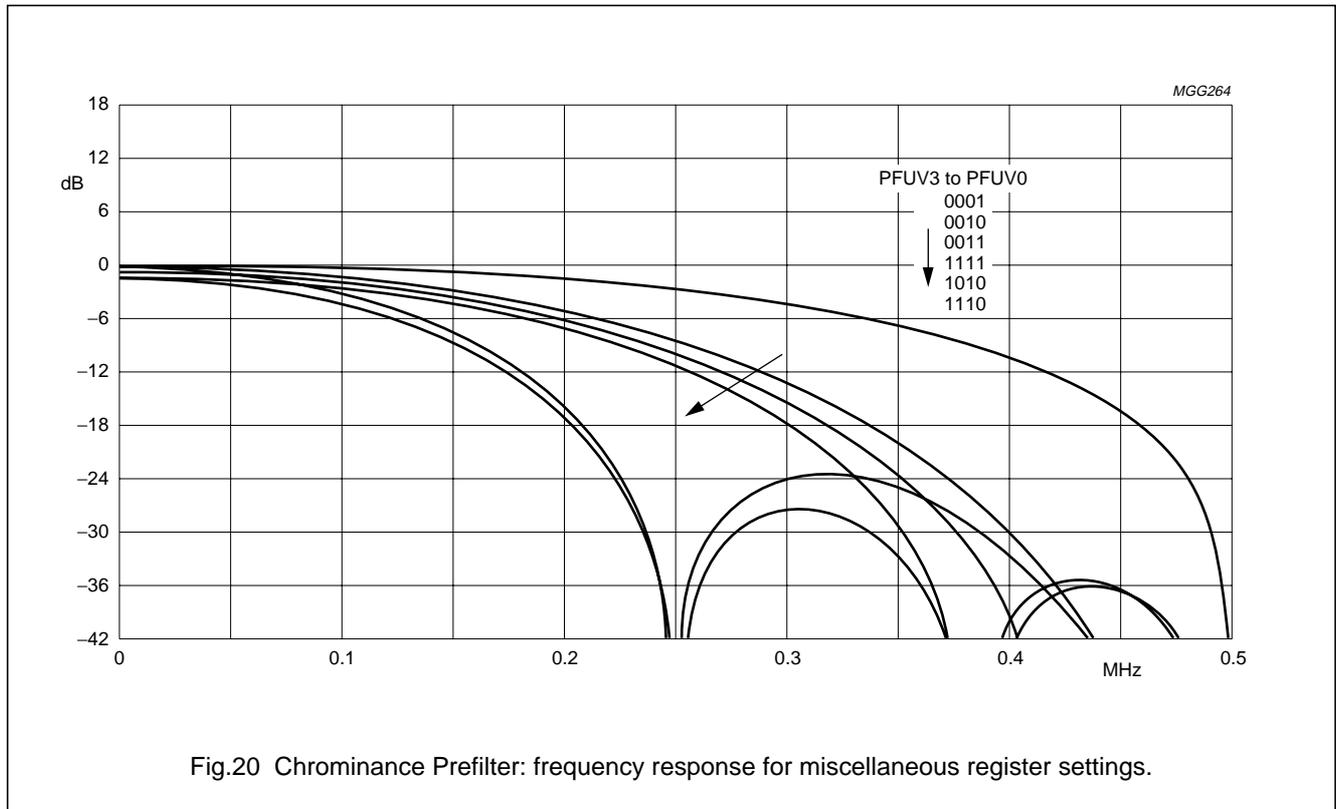
Fig.20 Chrominance Prefilter: frequency response for miscellaneous register settings.
