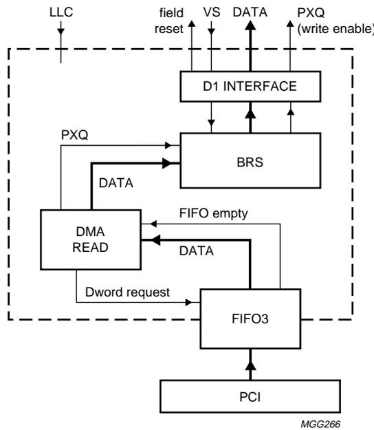
Fig.25 Sync and data path for field memory mode.
