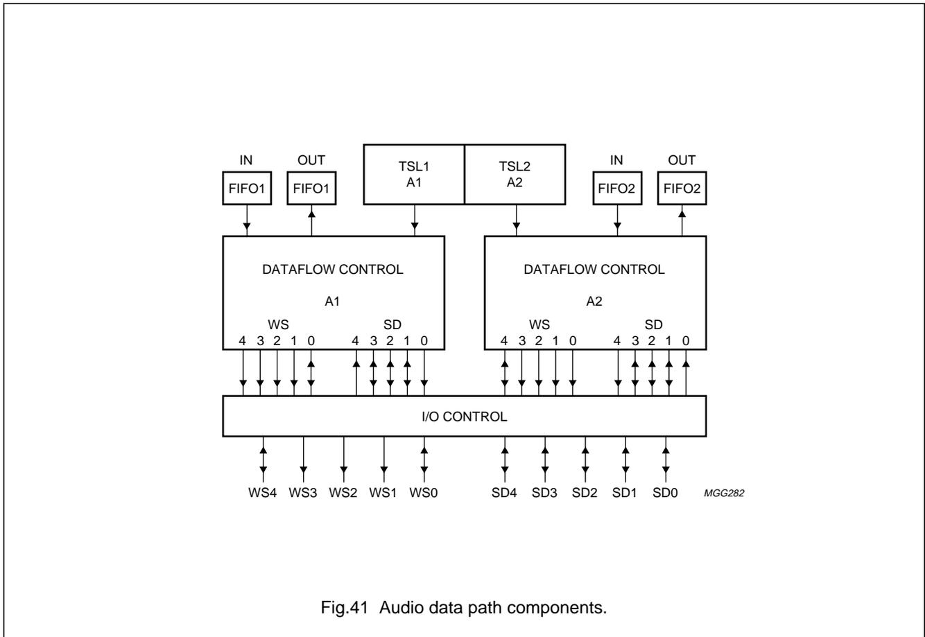
Fig.41 Audio data path components.
