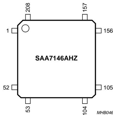
Fig.3 Pin configuration SAA7146AHZ (SQFP208).
