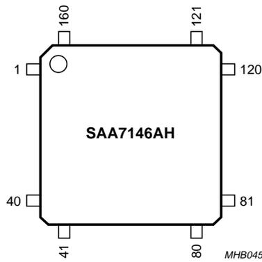
Fig.2 Pin configuration SAA7146AH (QFP160).
