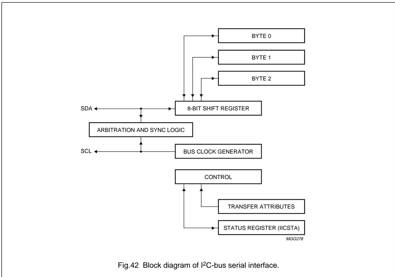
Fig.42 Block diagram of I<sup>2</sup>C-bus serial interface.
