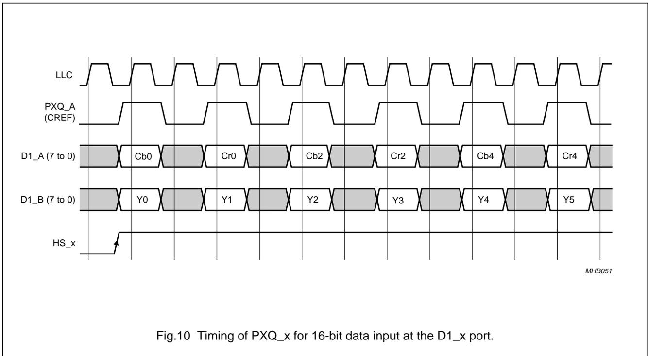
Fig.10 Timing of PXQ\_x for 16-bit data input at the D1\_x port.
