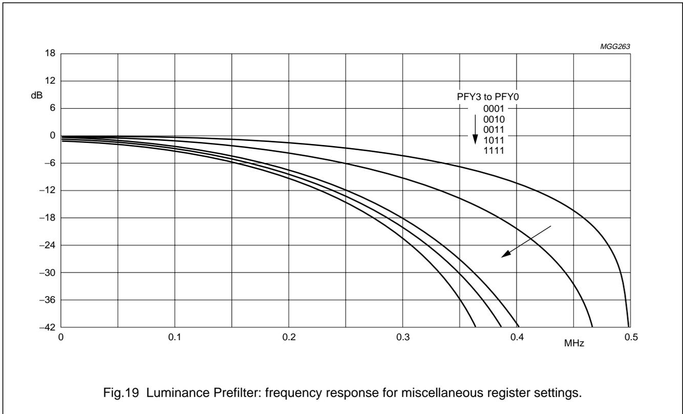
Fig.19 Luminance Prefilter: frequency response for miscellaneous register settings.
