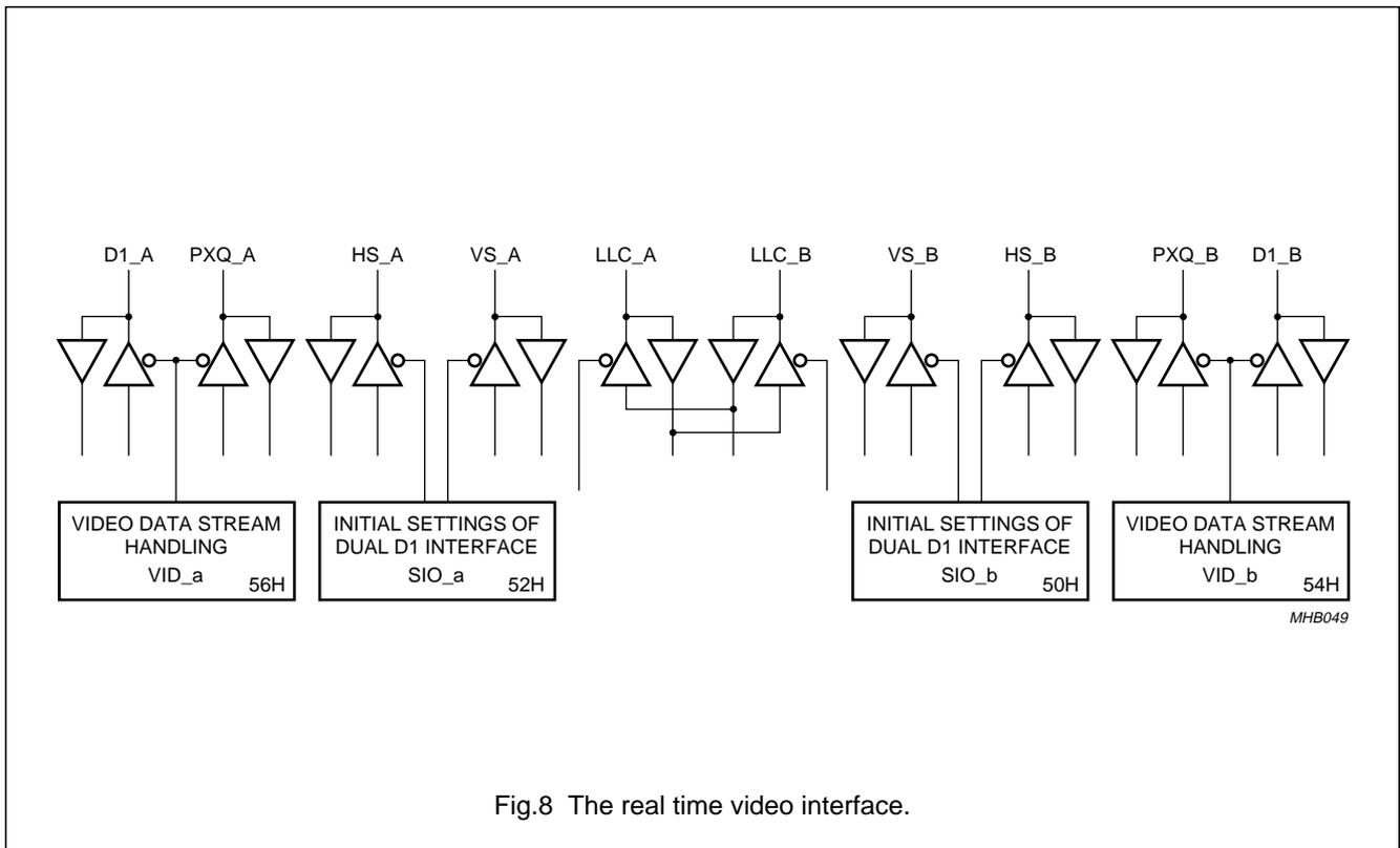
Fig.8 The real time video interface.
