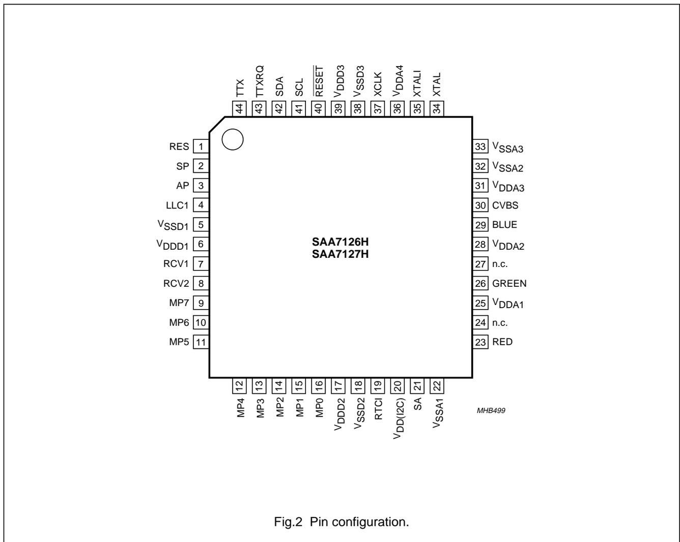
Fig.2 Pin configuration.
