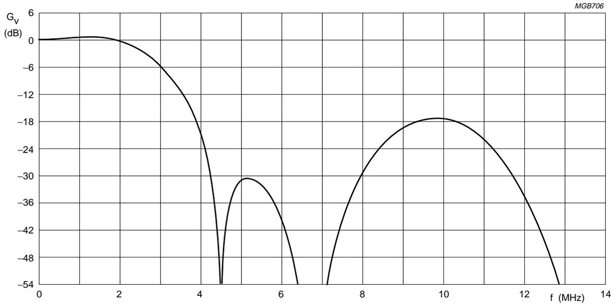
Fig.8 Colour difference transfer characteristic in RGB.
