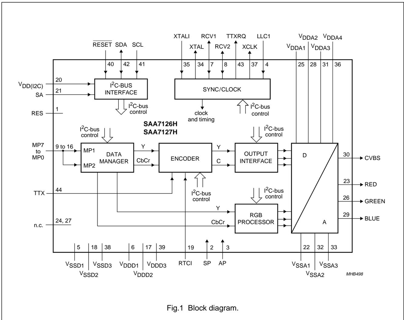
Fig.1 Block diagram.
