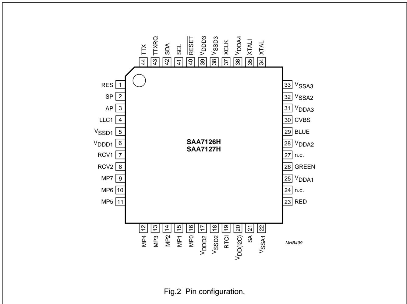
Fig.2 Pin configuration.
