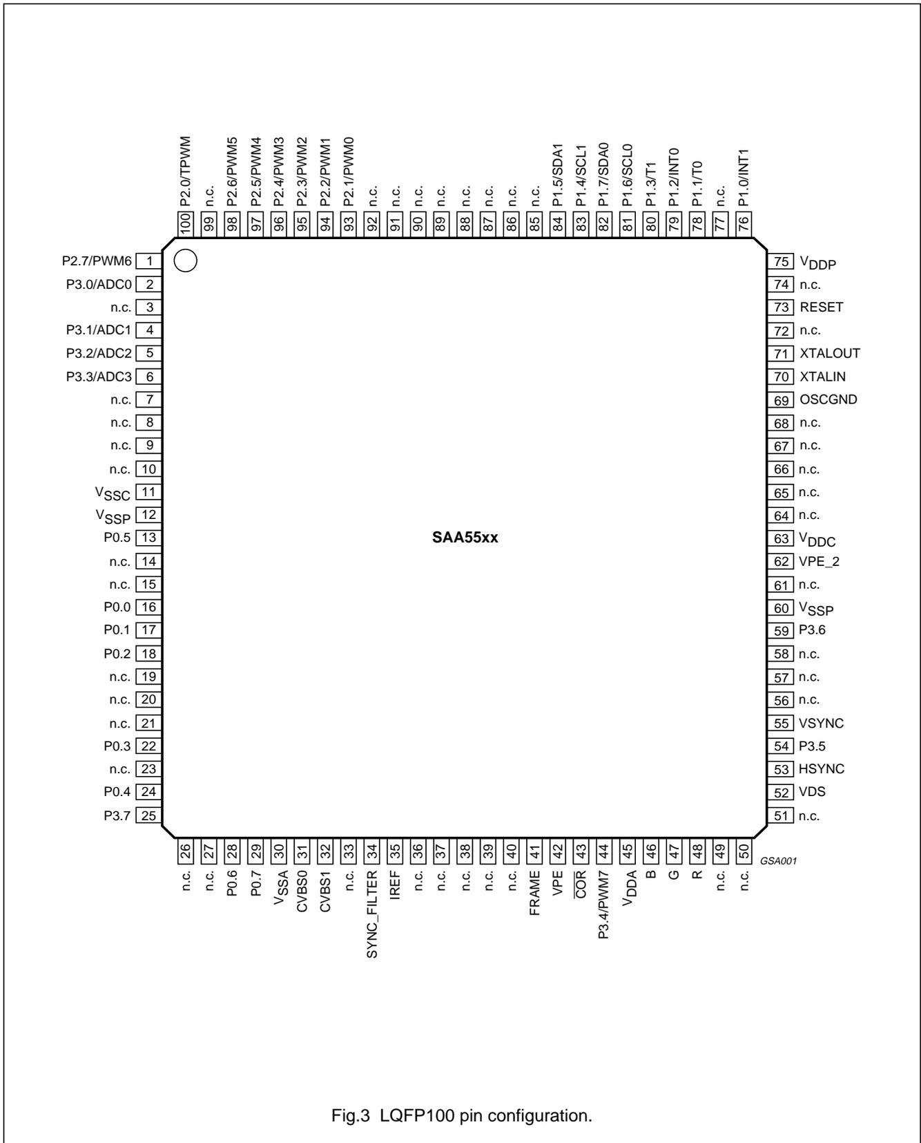
Fig.3 LQFP100 pin configuration.
