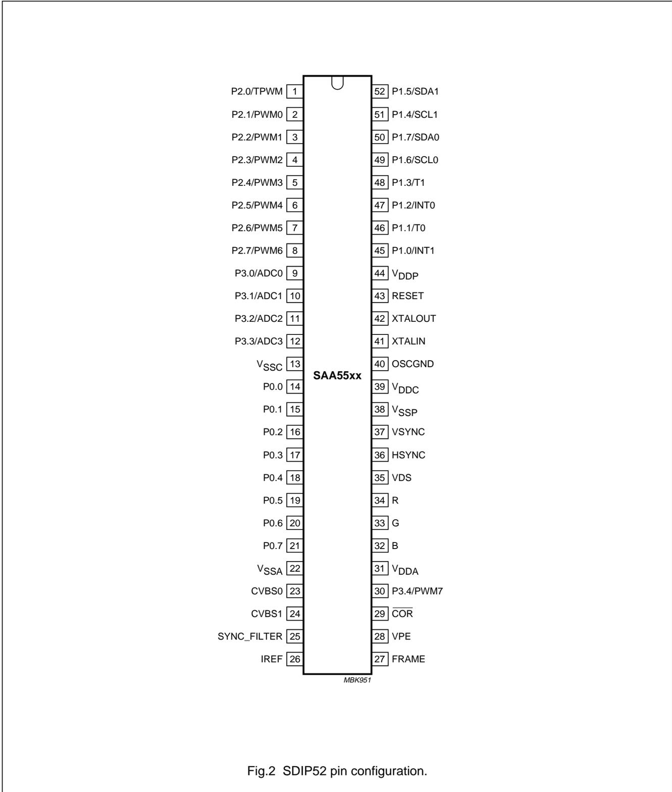
Fig.2 SDIP52 pin configuration.
