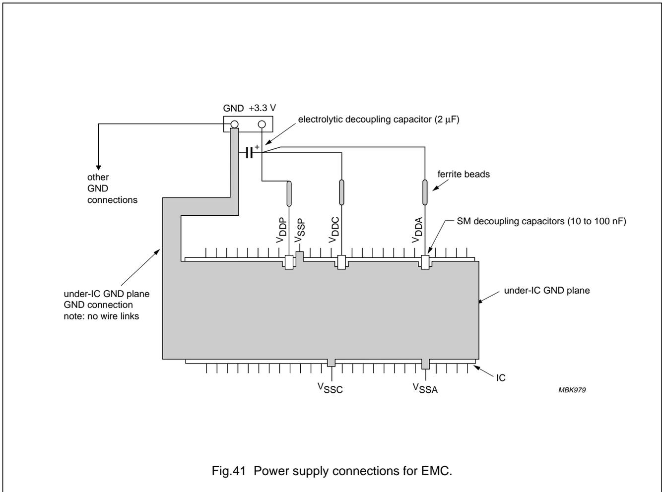
Fig.41 Power supply connections for EMC.
