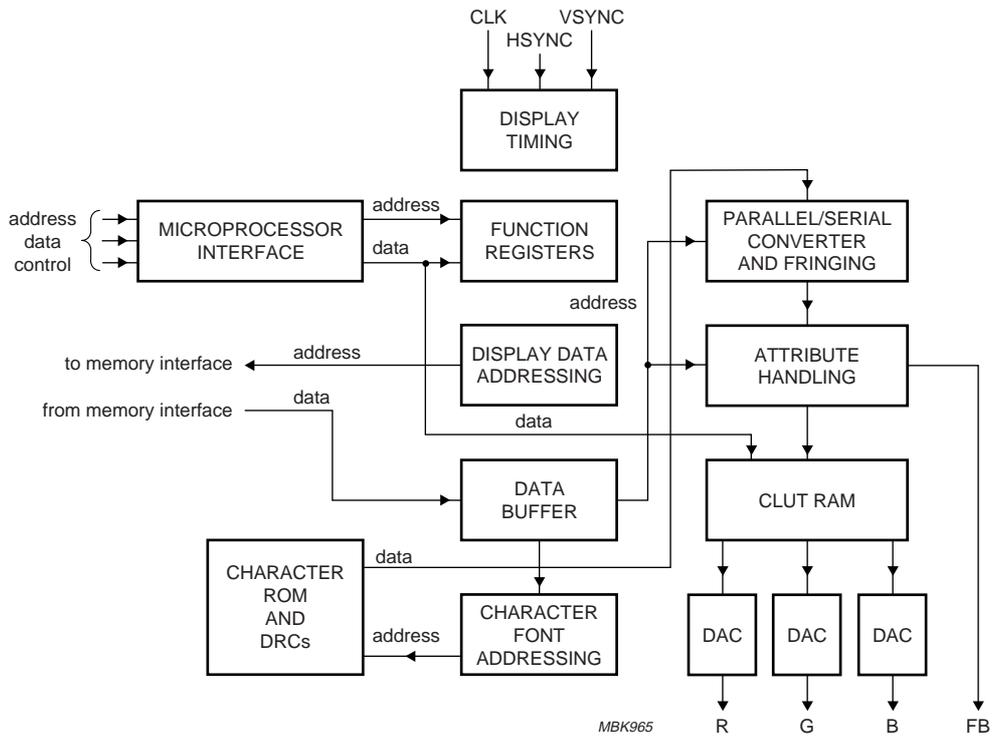
Fig.24 Display block diagram.
