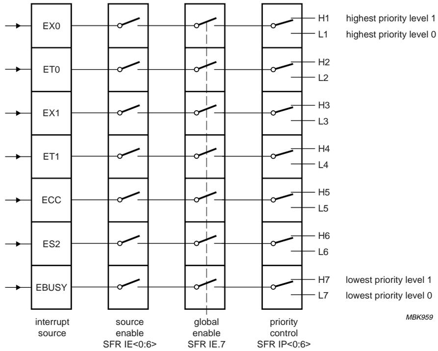
Fig.12 Interrupt structure.
