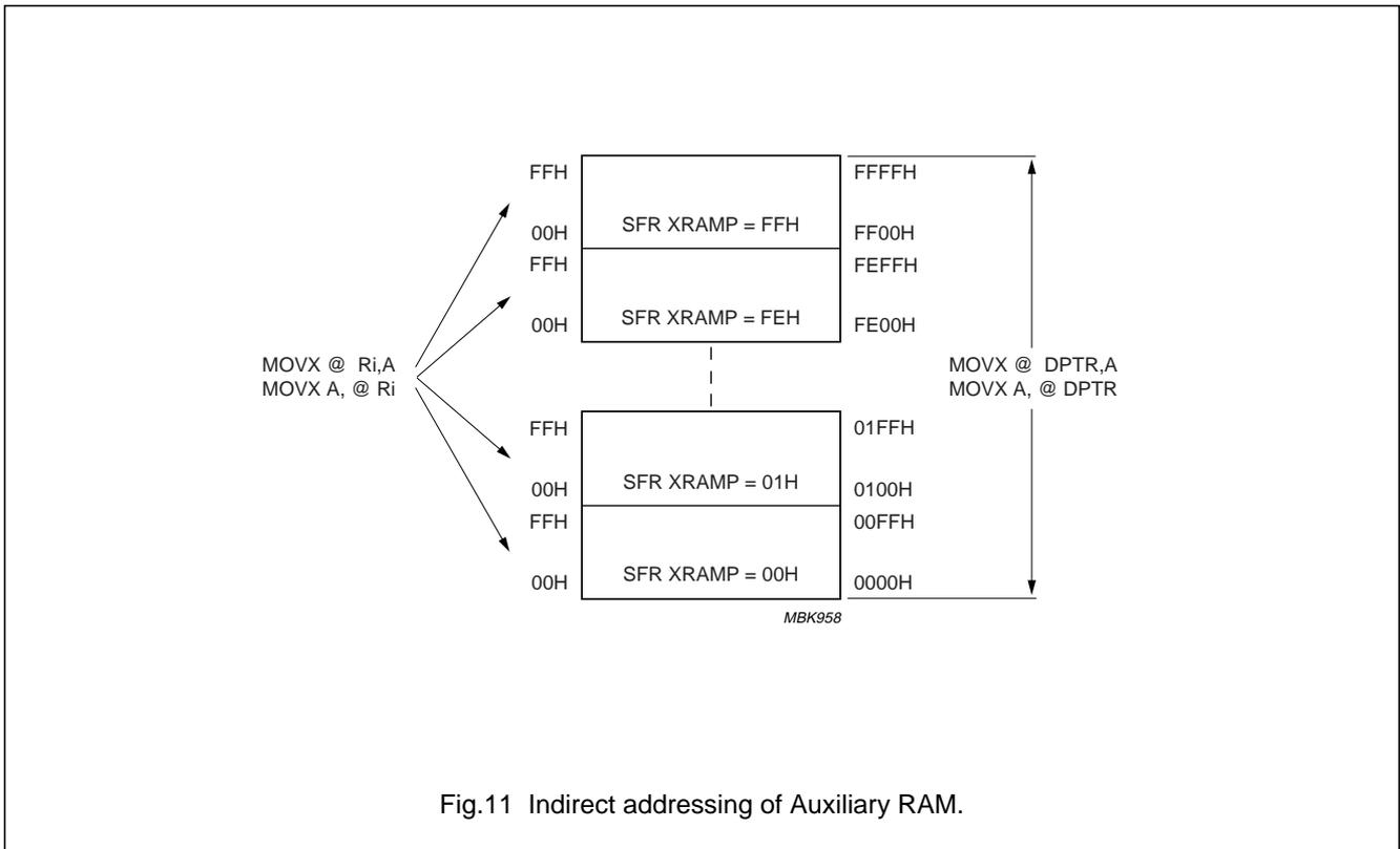
Fig.11 Indirect addressing of Auxiliary RAM.
