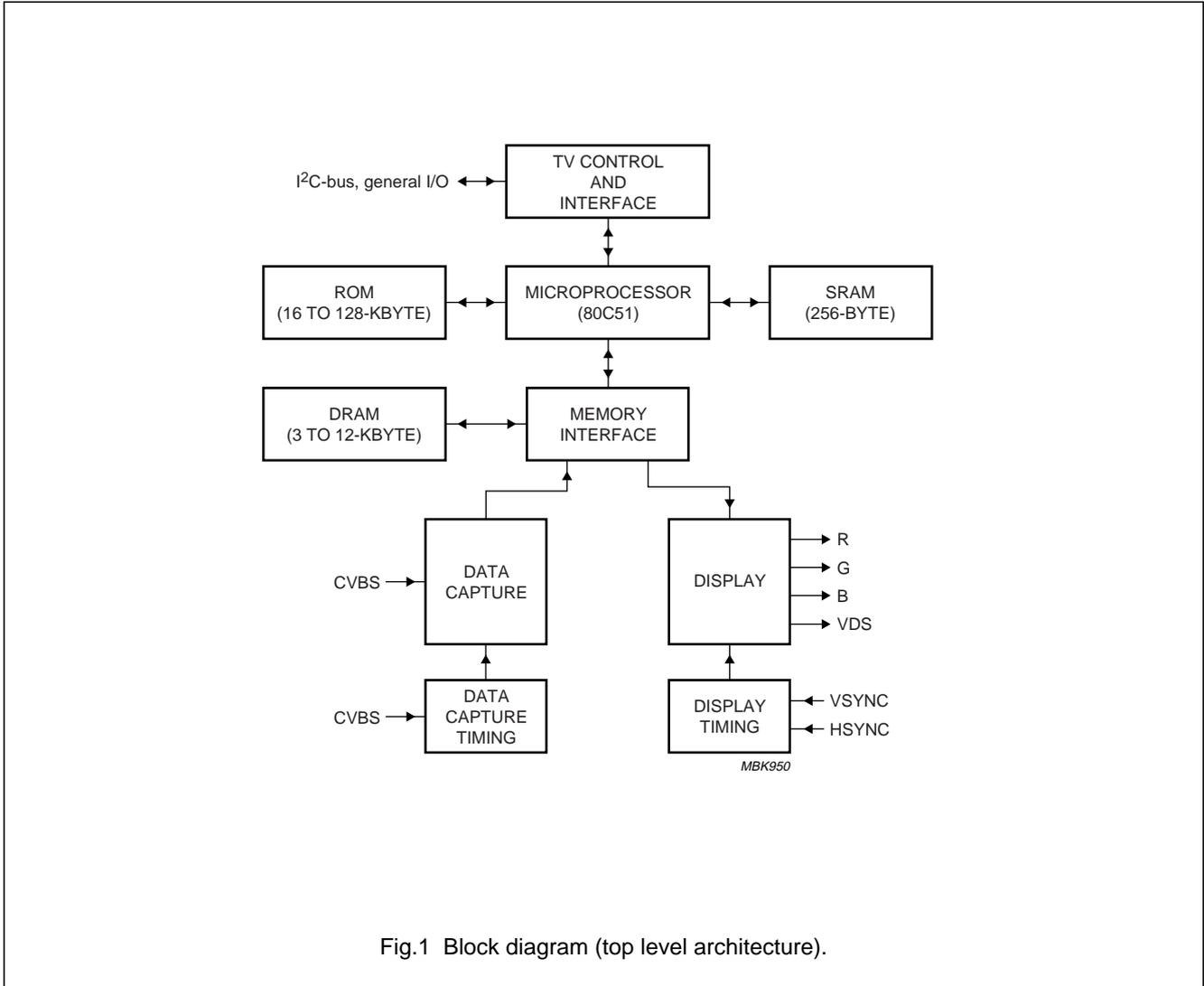
Fig.1 Block diagram (top level architecture).
