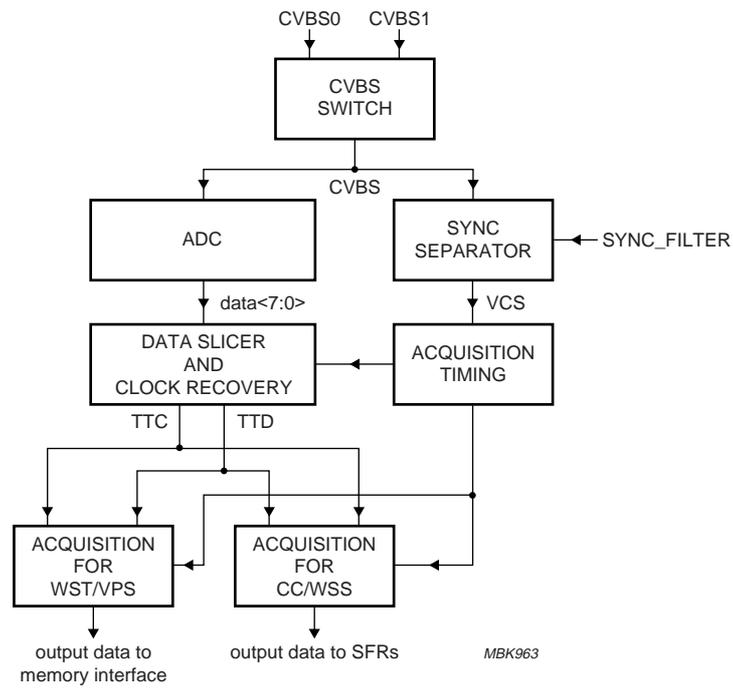
Fig.16 Data capture block diagram.
