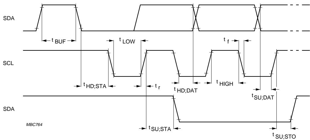
Fig.3 I<sup>2</sup>C-bus timing.
