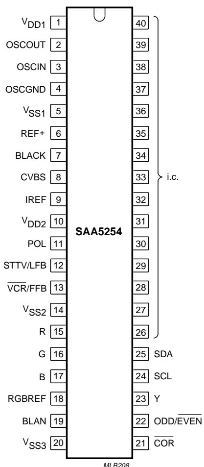
Fig.2 Pin configuration; SOT129 (DIP40).
