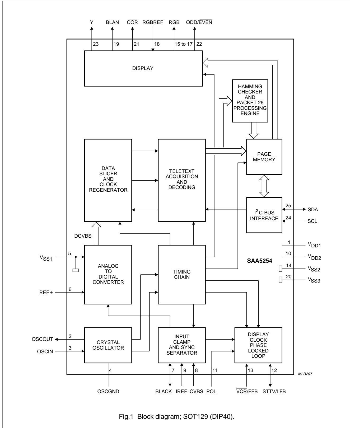
Fig.1 Block diagram; SOT129 (DIP40).
