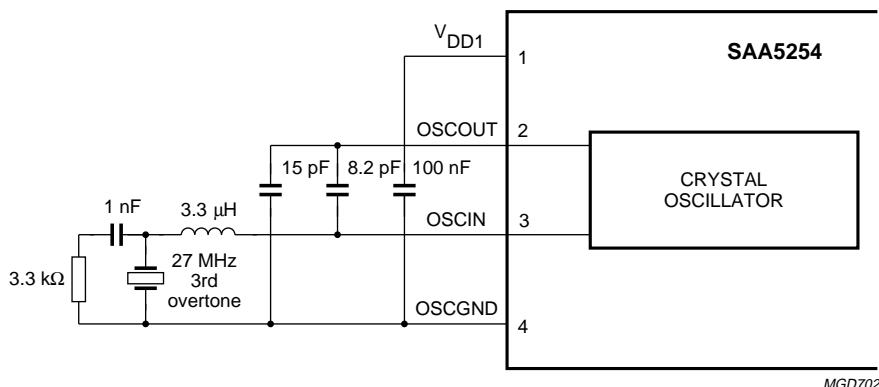
Fig.9 Crystal oscillator application diagram.
