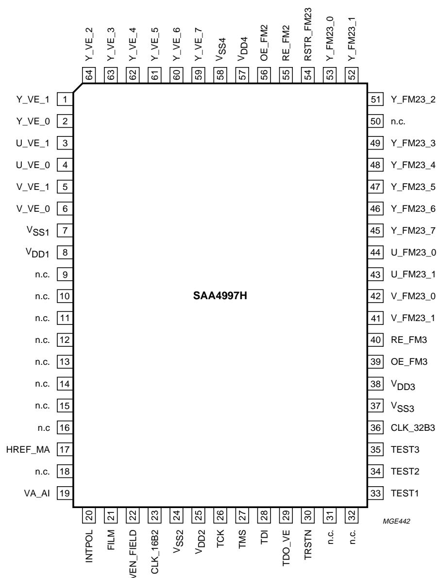
Fig.3 Pin configuration.
