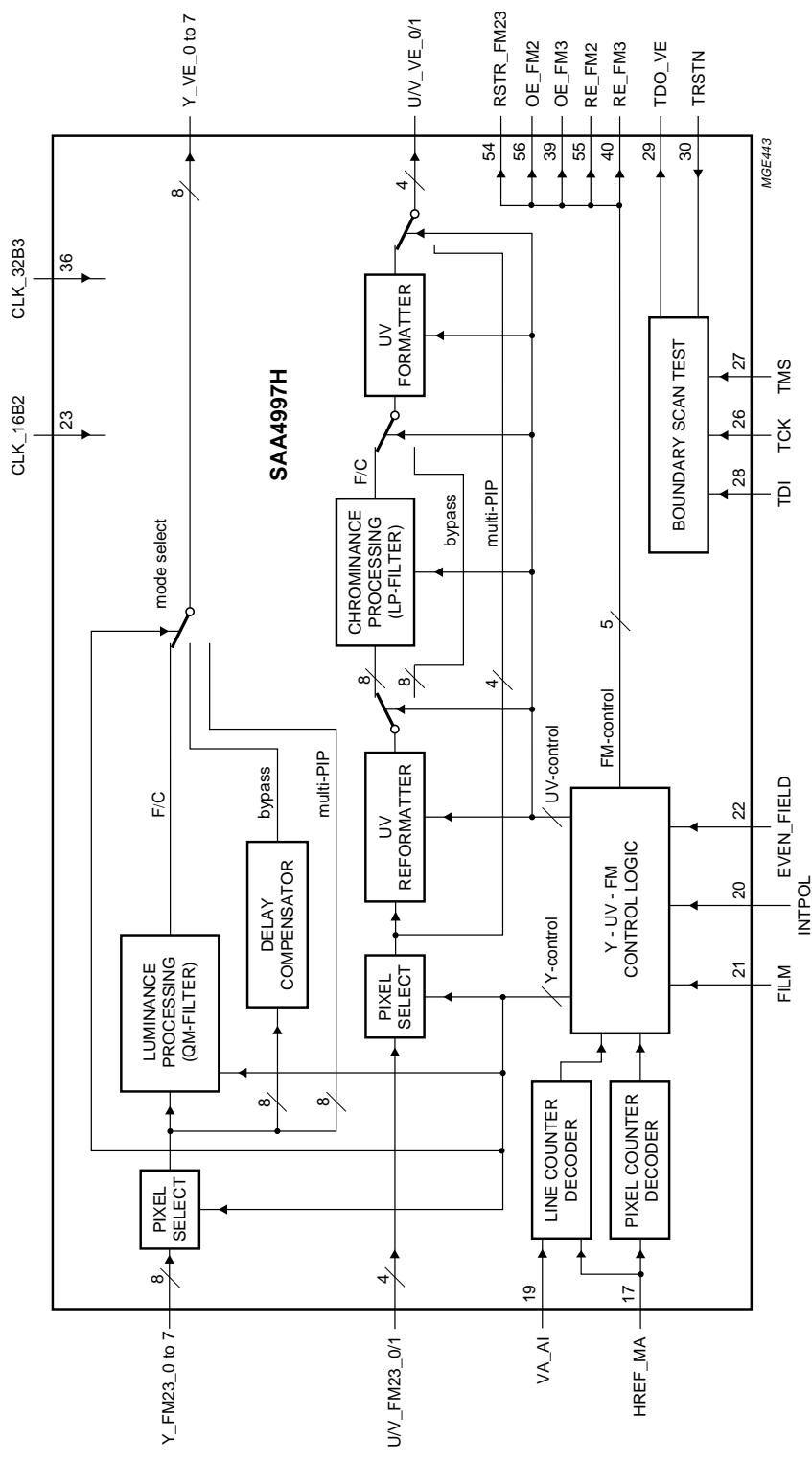
Fig.1 Block diagram.
