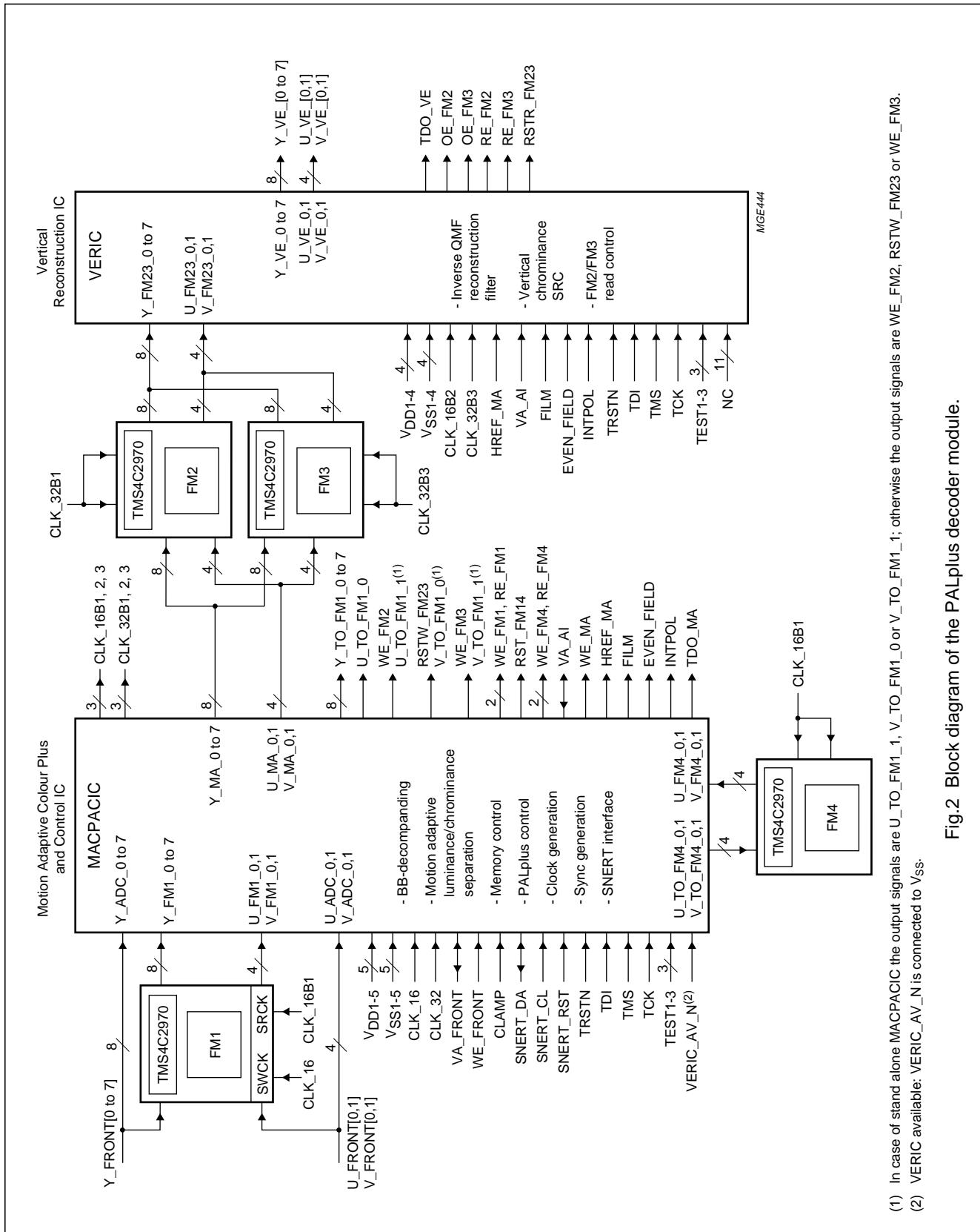
Fig.2 Block diagram of the PALplus decoder module.
