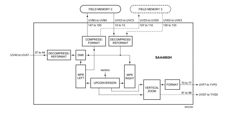
The solid lines represent pixel data; the broken lines represent the data flow, if the (optional) field memory 3 is also used.
