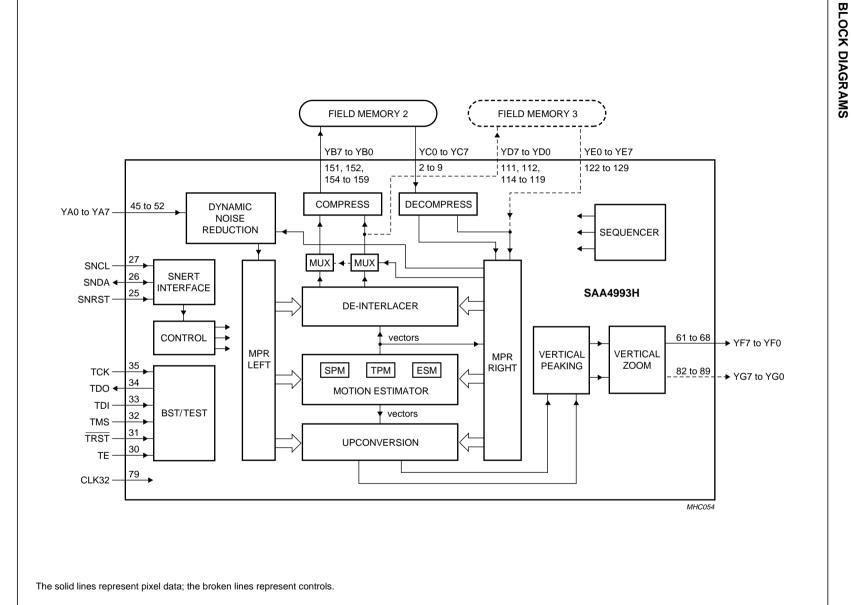
Fig.1 Block diagram of the luminance part.
