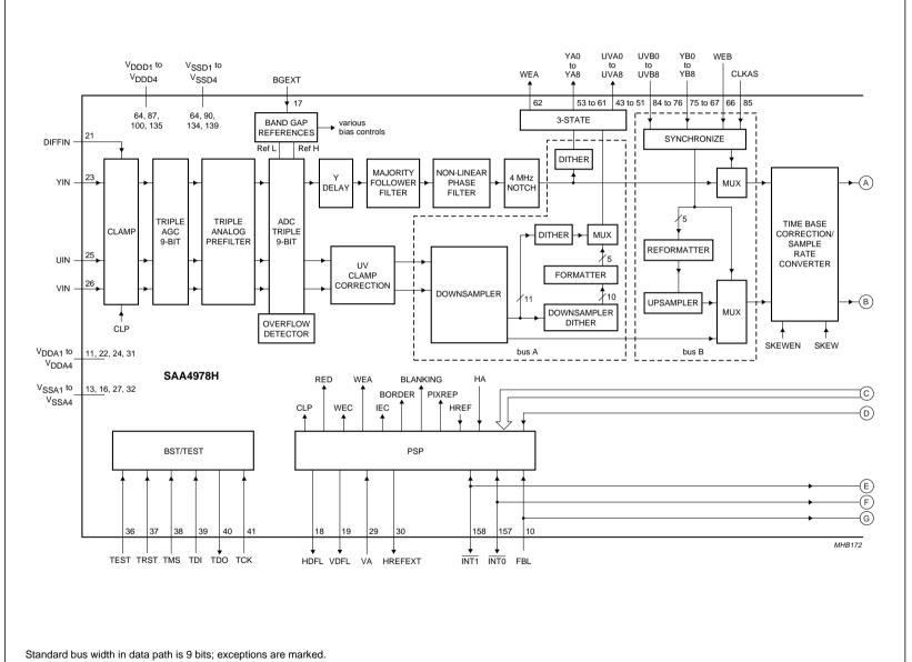
Fig.1 Block diagram (continued in Fig.2).
