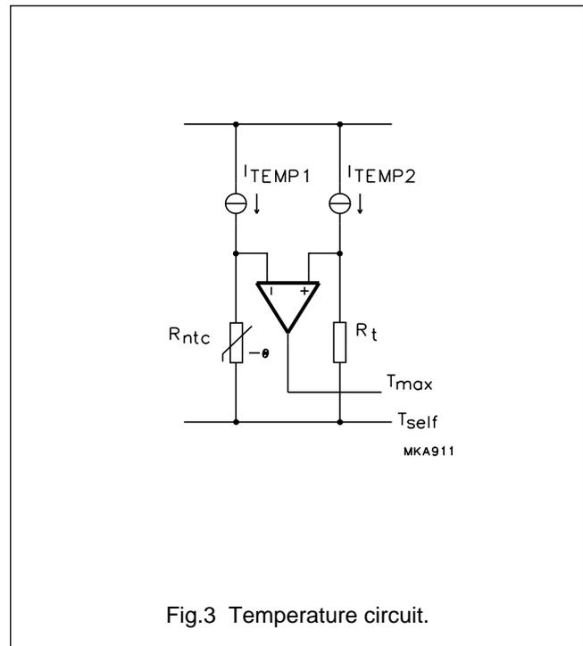
Fig.3 Temperature circuit.
