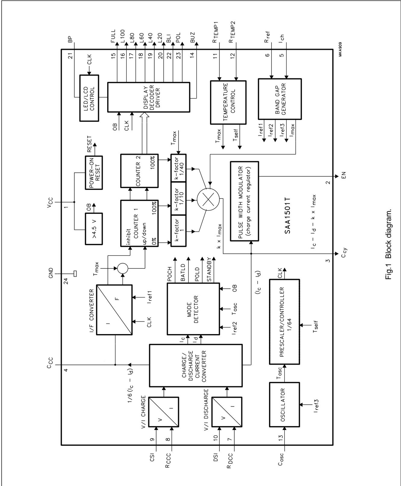
Fig.1 Block diagram.
