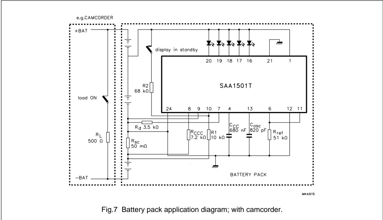
Fig.7 Battery pack application diagram; with camcorder.
