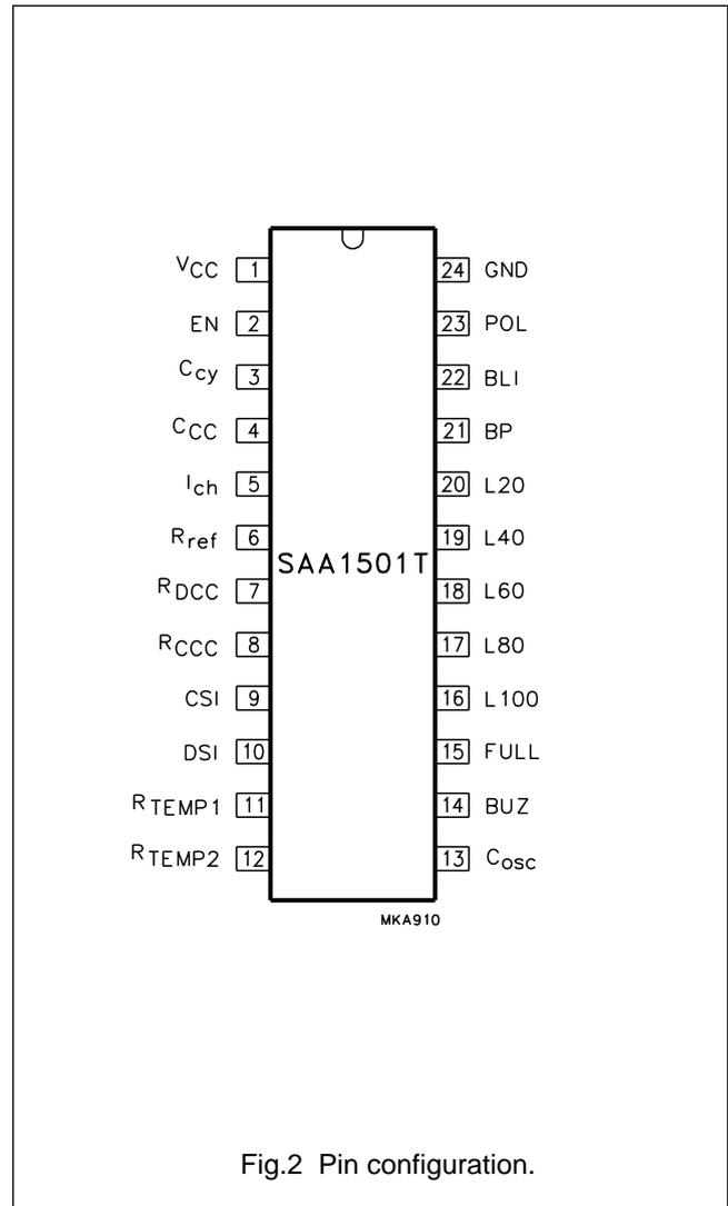
Fig.2 Pin configuration.
