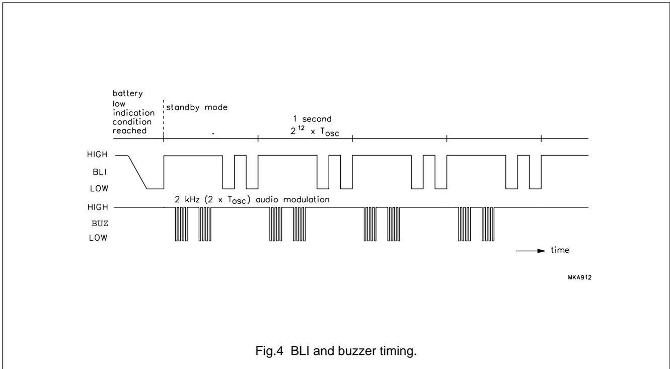
Fig.4 BLI and buzzer timing.
