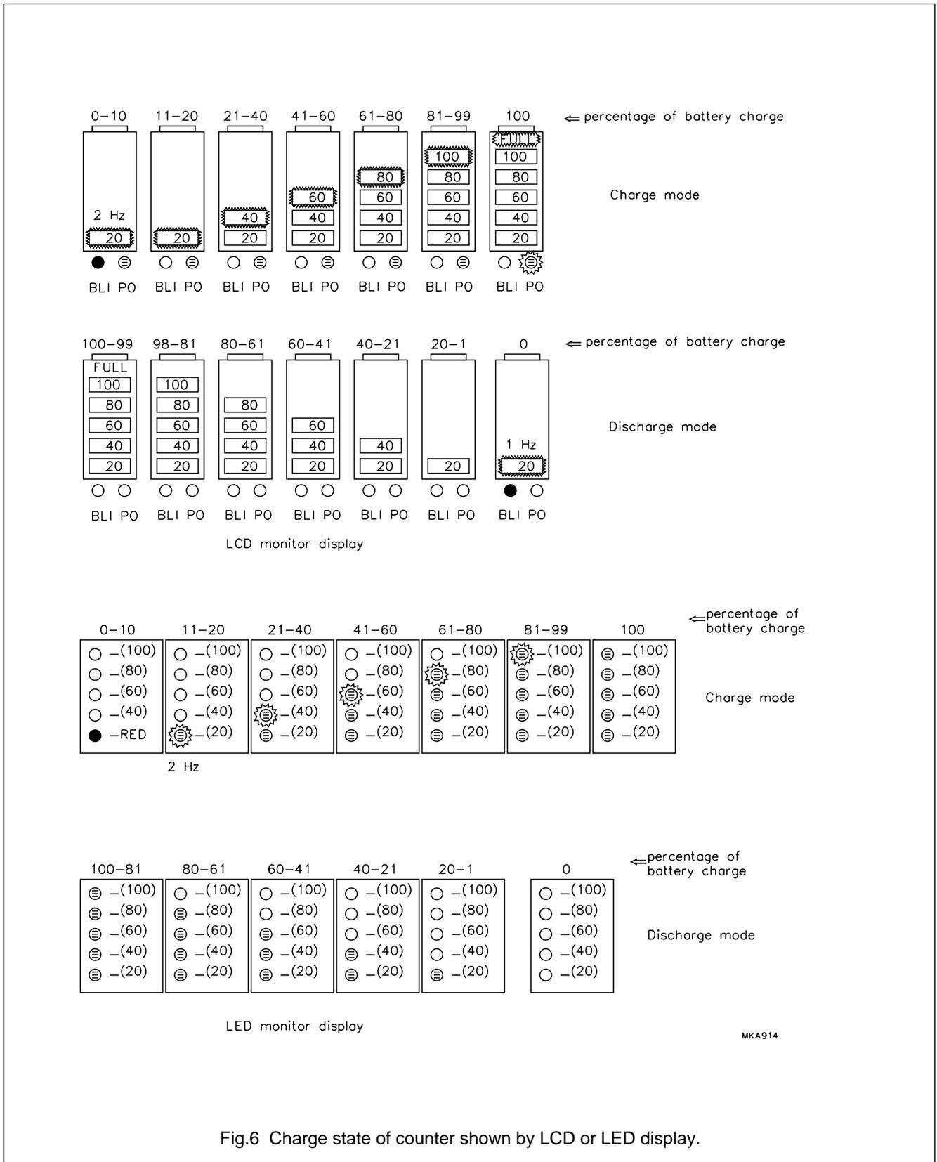
Fig.6 Charge state of counter shown by LCD or LED display.
