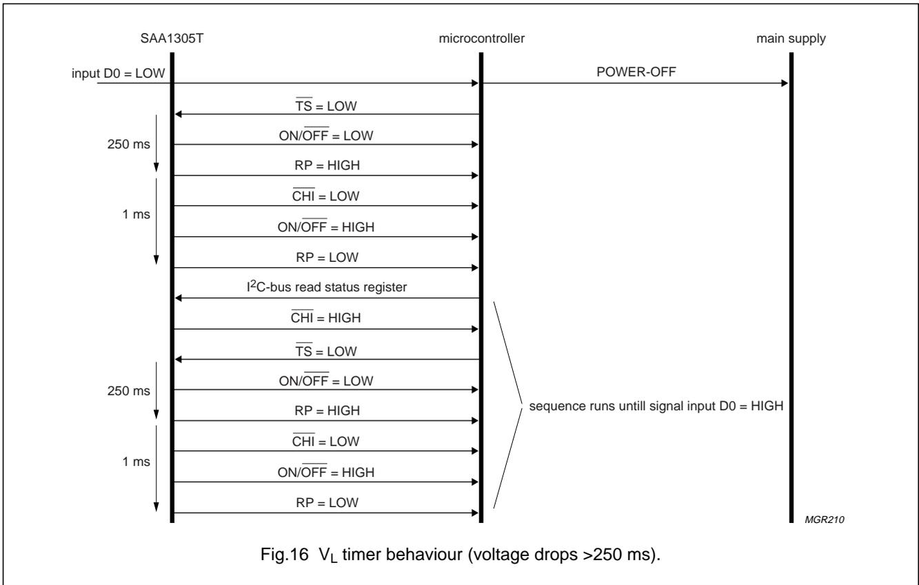
Fig.16 V<sub>L</sub> timer behaviour (voltage drops >250 ms).
