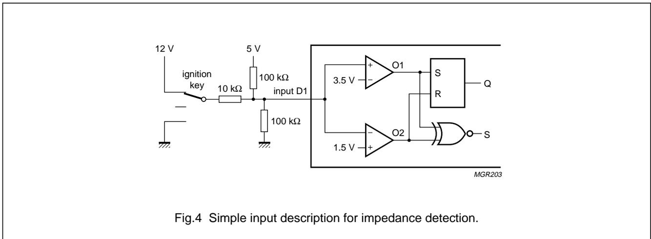
Fig.4 Simple input description for impedance detection.
