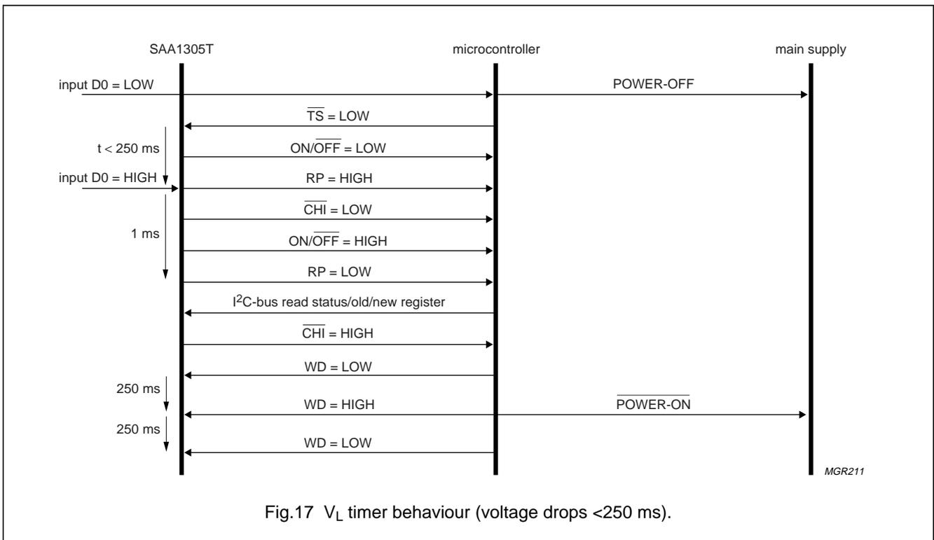
Fig.17 V<sub>L</sub> timer behaviour (voltage drops <250 ms).
