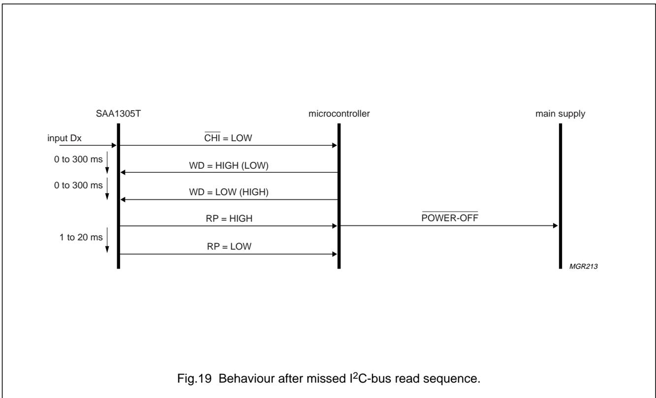
Fig.19 Behaviour after missed I<sup>2</sup>C-bus read sequence.
