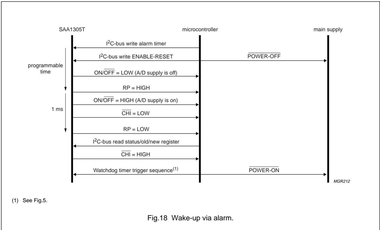
Fig.18 Wake-up via alarm.
