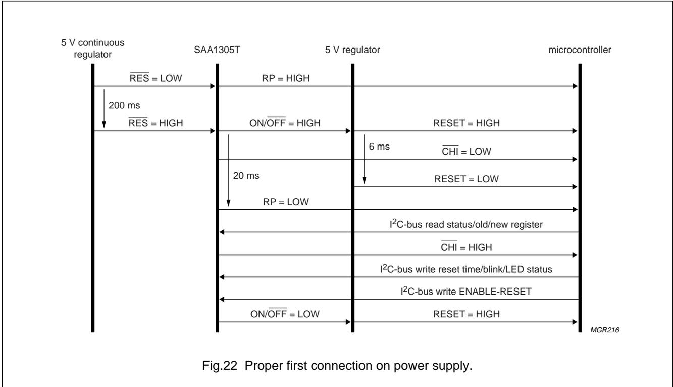
Fig.22 Proper first connection on power supply.
