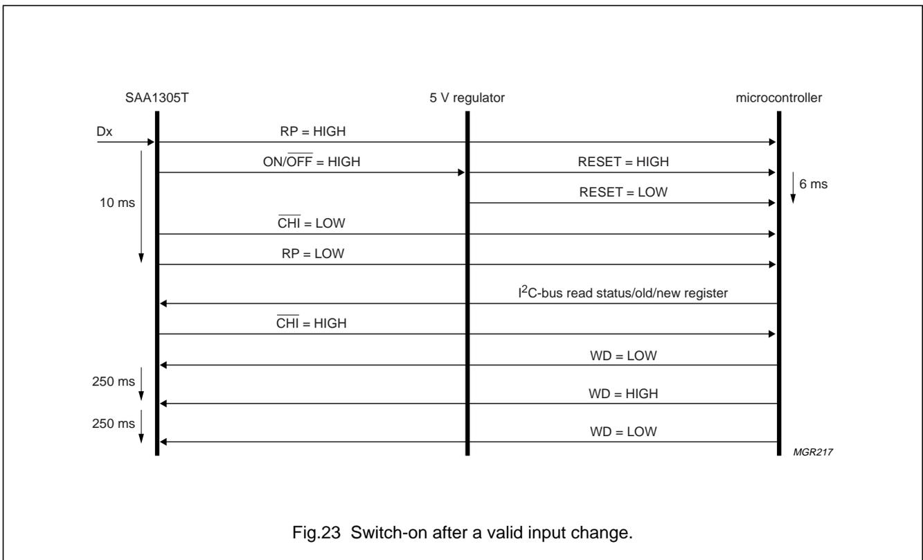
Fig.23 Switch-on after a valid input change.
