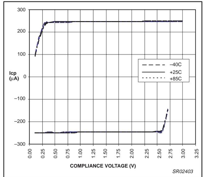
Figure 26. PHA charge pump output vs. temperature
