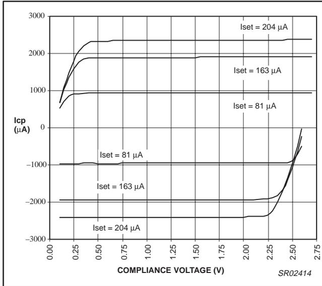
Figure 11. PHI\_SU charge pump output vs. Iset
