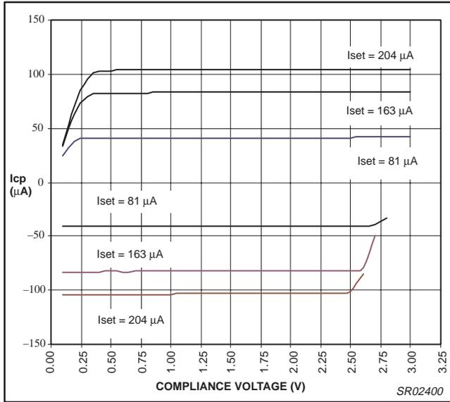
Figure 23. PHA charge pump output vs. Iset
