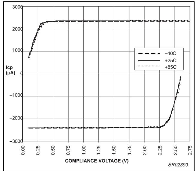
Figure 22. PHP\_SU charge pump output vs. temperature
