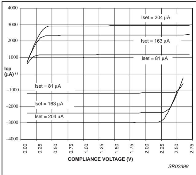
Figure 21. PHP\_SU charge pump output vs. Iset
