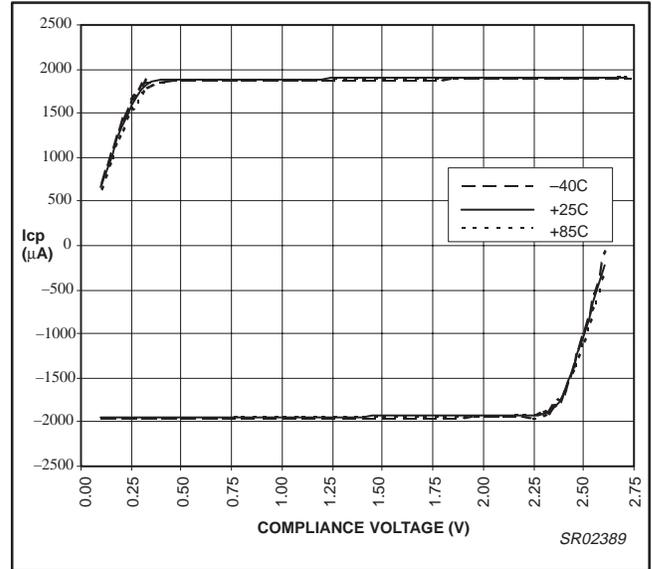
Figure 12. PHI\_SU charge pump output vs. temperature
