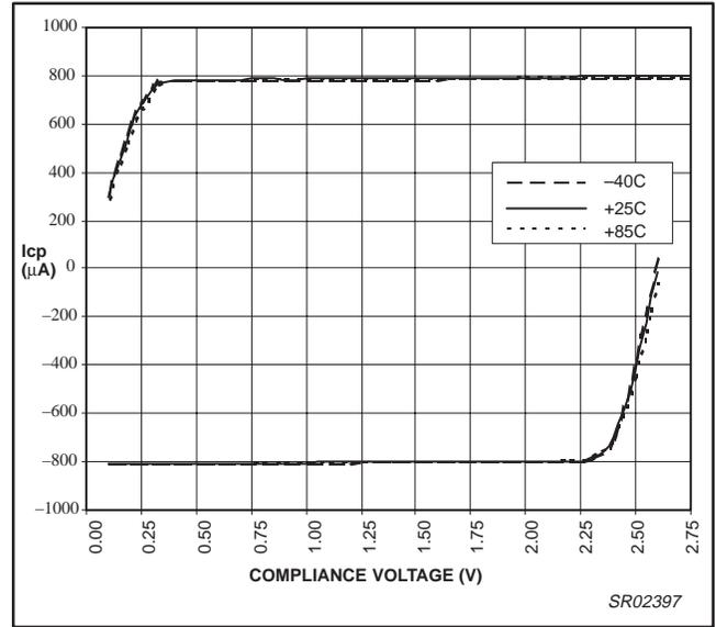
Figure 20. PHP\_SU charge pump output vs. temperature
