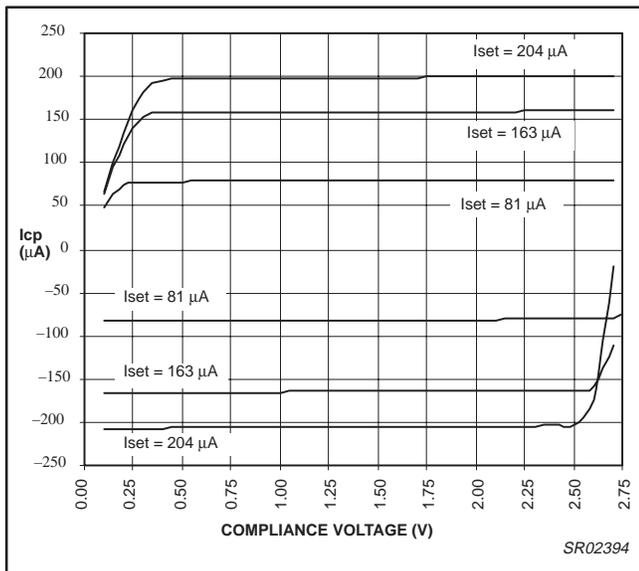
Figure 17. PHP charge pump output vs. Iset
