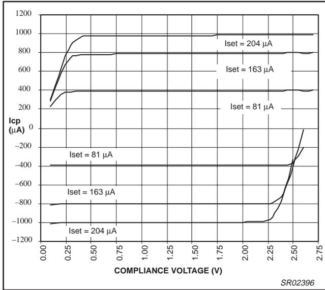
Figure 19. PHP\_SU charge pump output vs. Iset
