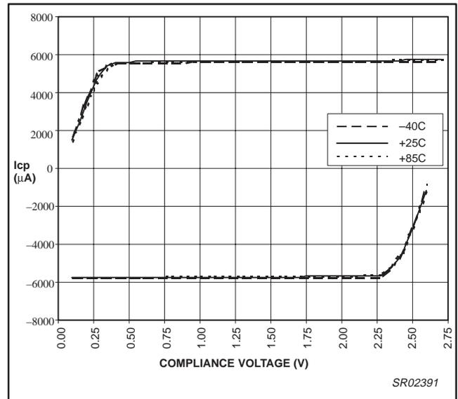
Figure 14. PHI\_SU charge pump output vs. temperature
