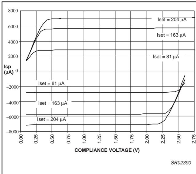
Figure 13. PHI\_SU charge pump output vs. Iset
