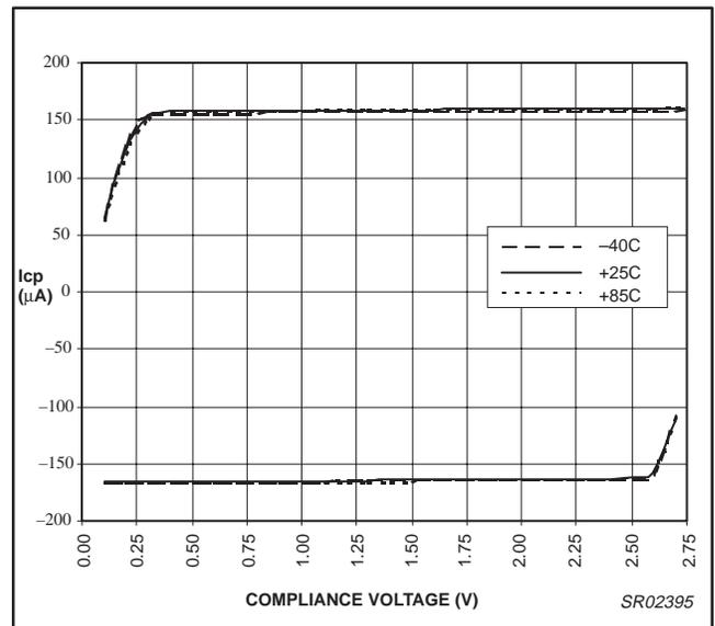
Figure 18. PHP charge pump output vs. temperature
