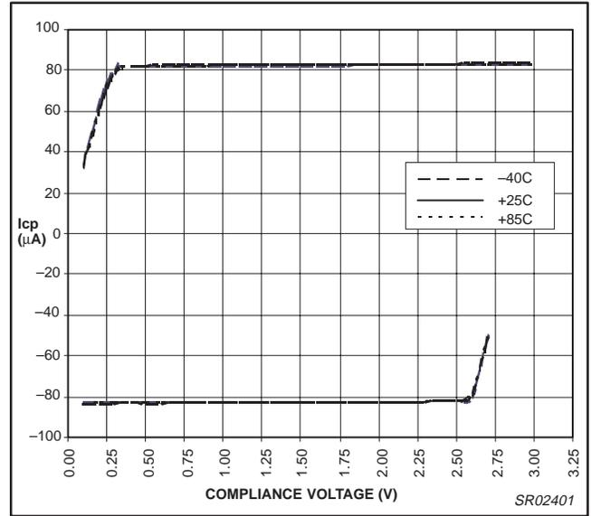
Figure 24. PHA charge pump output vs. temperature
