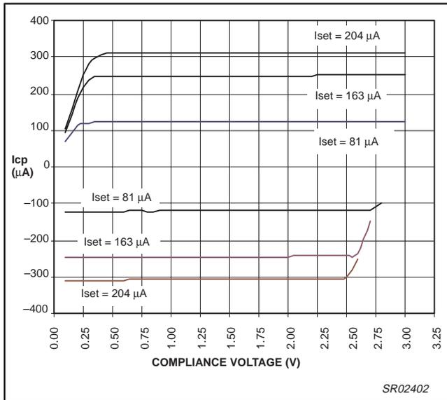
Figure 25. PHA charge pump output vs. Iset
