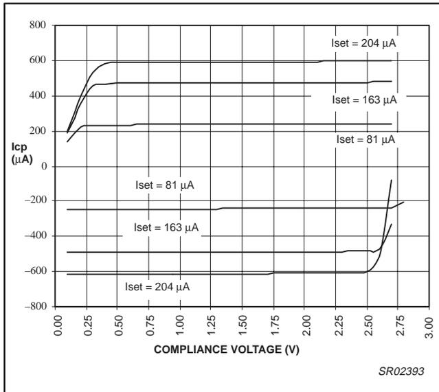
Figure 15. PHP charge pump output vs. Iset
