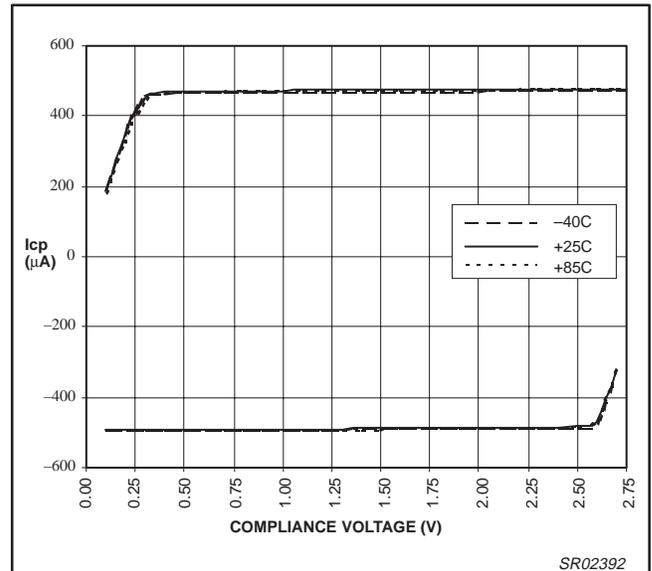
Figure 16. PHP charge pump output vs. temperature
