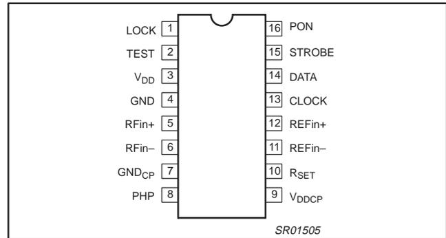
Figure 1. Pin Configuration
