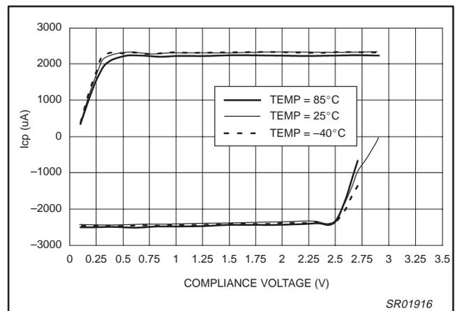
**Figure 14. Php-su Charge Pump Output vs. Temperature (CP = 0; V<sub>DD</sub> = 3.0 V; I<sub>SET</sub> = 165.33 uA)**
