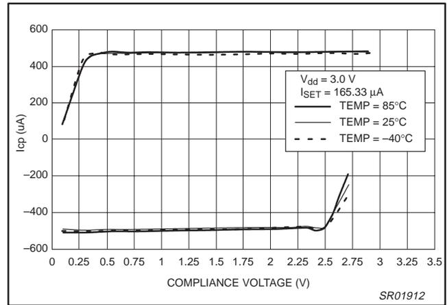
**Figure 10. Php Charge Pump Output vs. Temperature (CP = 0; V<sub>DD</sub> = 3.0 V; I<sub>SET</sub> = 165.33 uA)**
