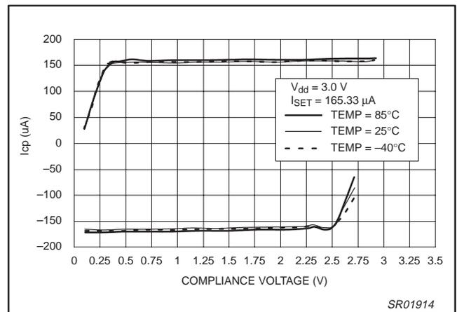
**Figure 12. Php Charge Pump Output vs. Temperature (CP = 1; V<sub>DD</sub> = 3.0 V; I<sub>SET</sub> = 165.33 uA)**
