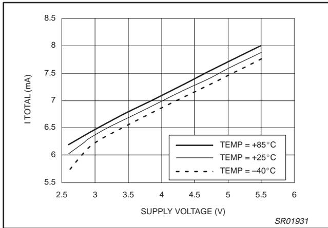
Figure 21. Current Supply Over V<sub>DD</sub>
