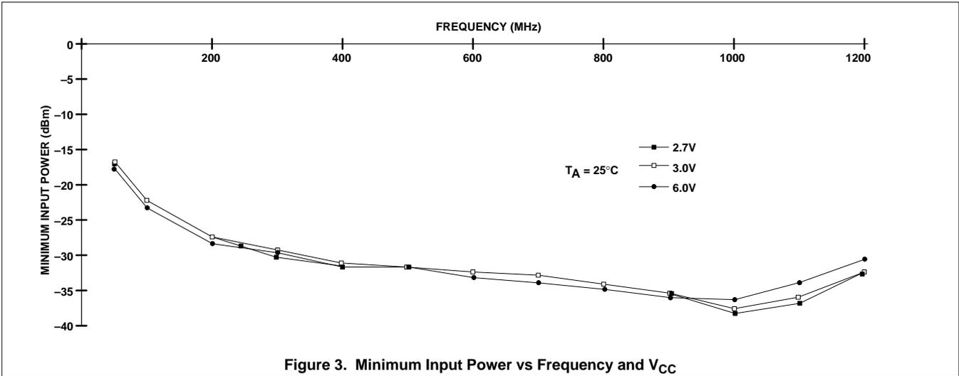
Figure 3. Minimum Input Power vs Frequency and V<sub>CC</sub>
