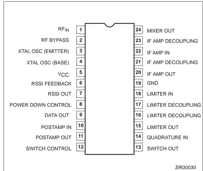
Figure 1. Pin Configuration
