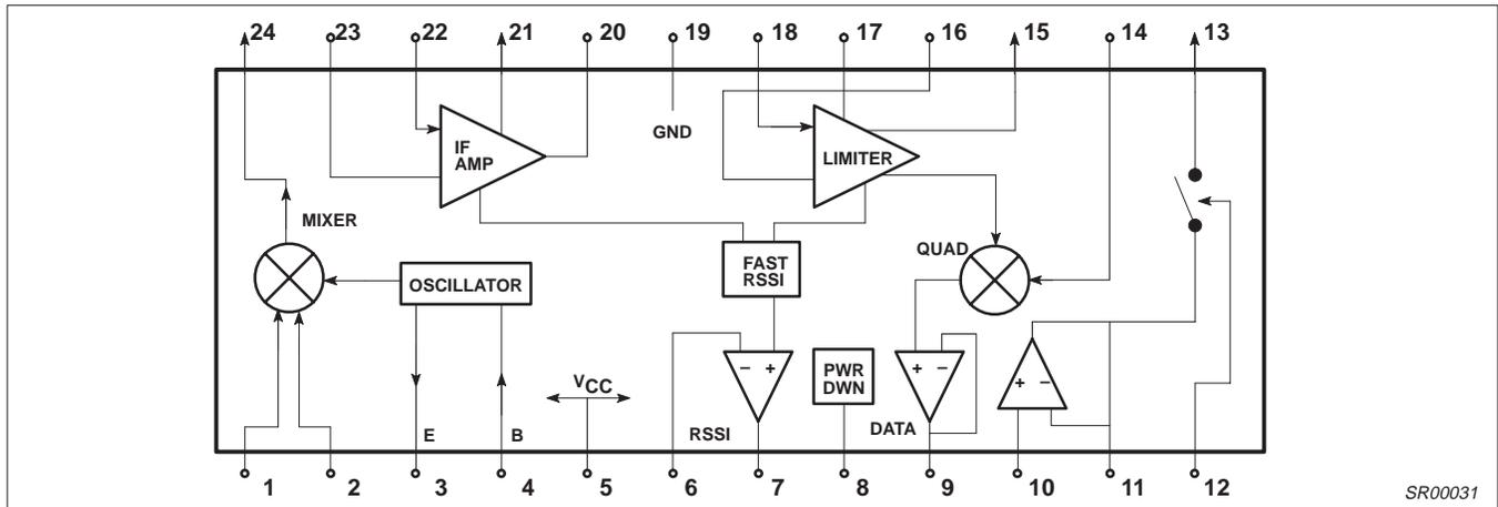
Figure 2. Block Diagram
