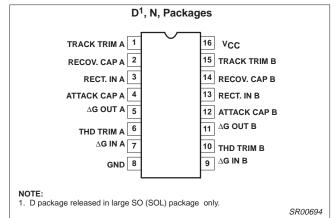
Figure 1. Pin Configuration
