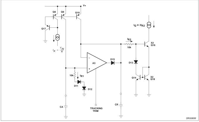
Figure 6. Buffer Amplifier Schematic
