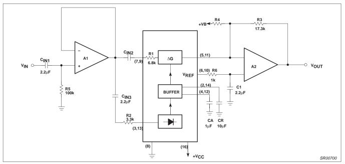
Figure 7. Basic Expandor Schematic
