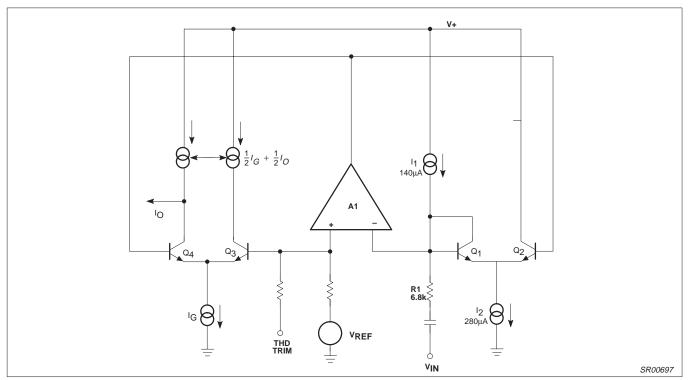
Figure 4. Basic Gain Cell Schematic
