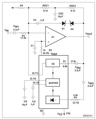
Figure 8. Basic Compressor Schematic
