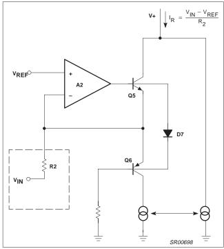
Figure 5. Simplified Rectifier Schematic
