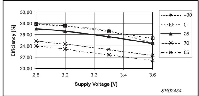
Figure 23. Efficiency vs. supply voltage, mode = high
