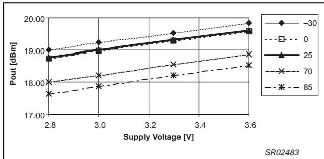
Figure 22. Output power vs. supply voltage, mode = high
