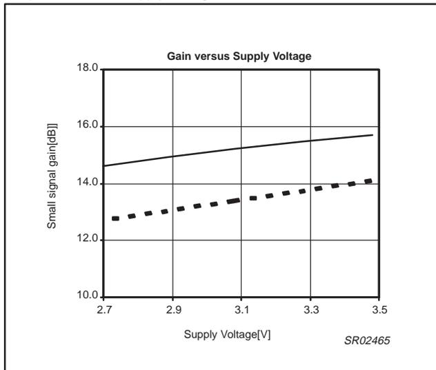
Figure 4. Gain vs. supply voltage
