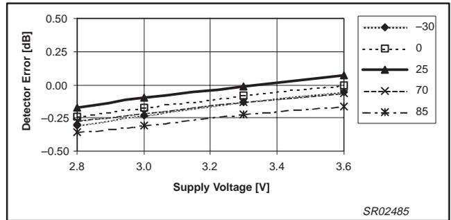
Figure 24. Detector error vs. supply voltage, mode = high
