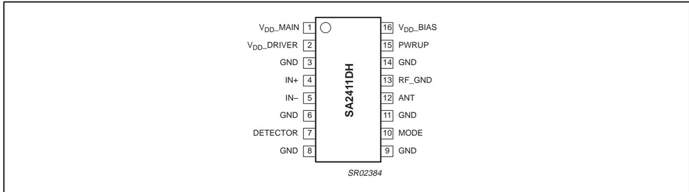
Figure 2. Pin configuration
