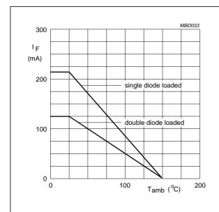
Device mounted on an FR4 printed-circuit board.
