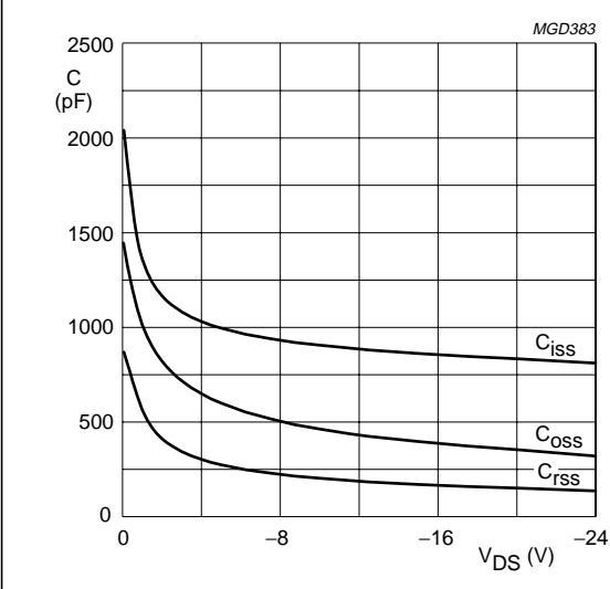
$V_{GS} = 0; f = 1 \text{ MHz}; T_j = 25^\circ\text{C}$ .
