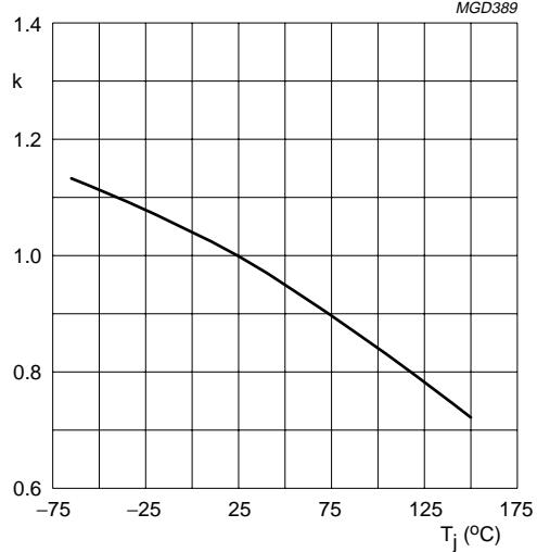
$$k = \frac{V_{GSth} \text{ at } T_j}{V_{GSth} \text{ at } 25^\circ\text{C}}$$
