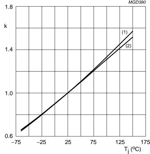
$$k = \frac{R_{DSon} \text{ at } T_j}{R_{DSon} \text{ at } 25^\circ\text{C}}$$
