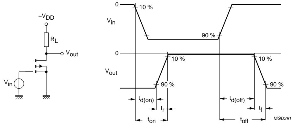
Fig.11 Switching times test circuit and input and output waveforms.
