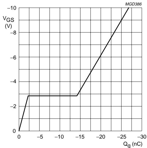
$V_{DD} = -15 \text{ V}; I_D = -2.5 \text{ A.}$
