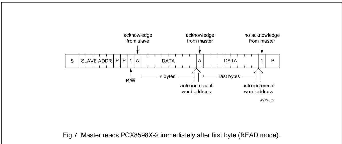
Fig.7 Master reads PCX8598X-2 immediately after first byte (READ mode).
