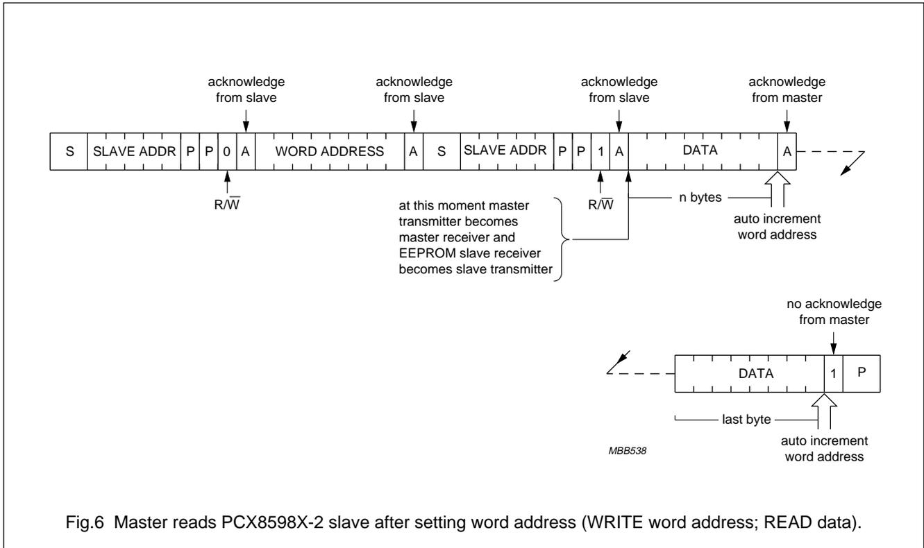
Fig.6 Master reads PCX8598X-2 slave after setting word address (WRITE word address; READ data).
