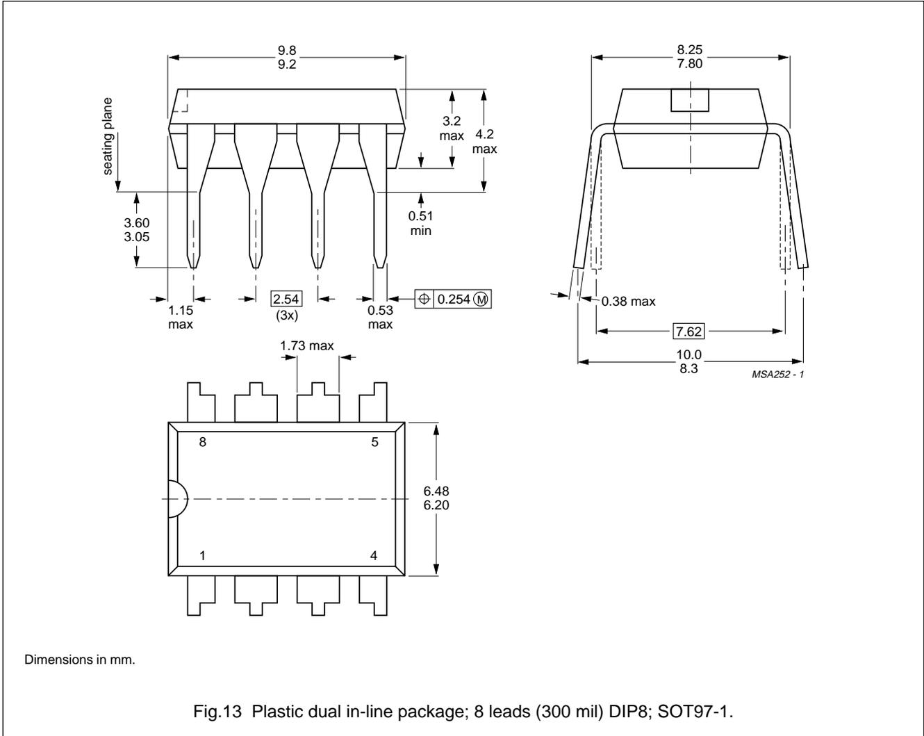
Fig.13 Plastic dual in-line package; 8 leads (300 mil) DIP8; SOT97-1.
