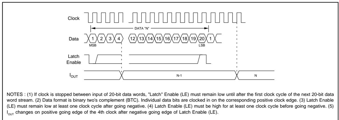
FIGURE 2. Timing Diagram.
