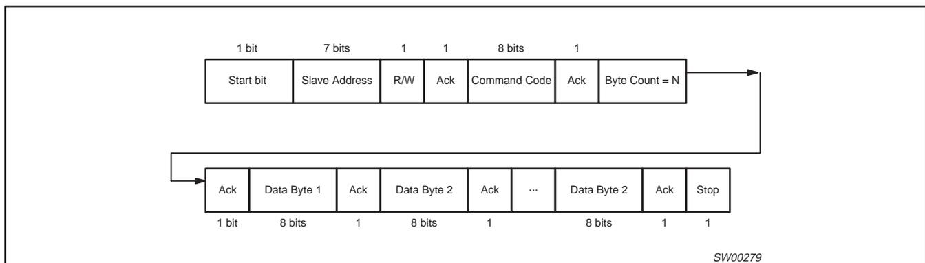
**NOTE:** The acknowledgement bit is returned by the slave/receiver (the clock driver).
