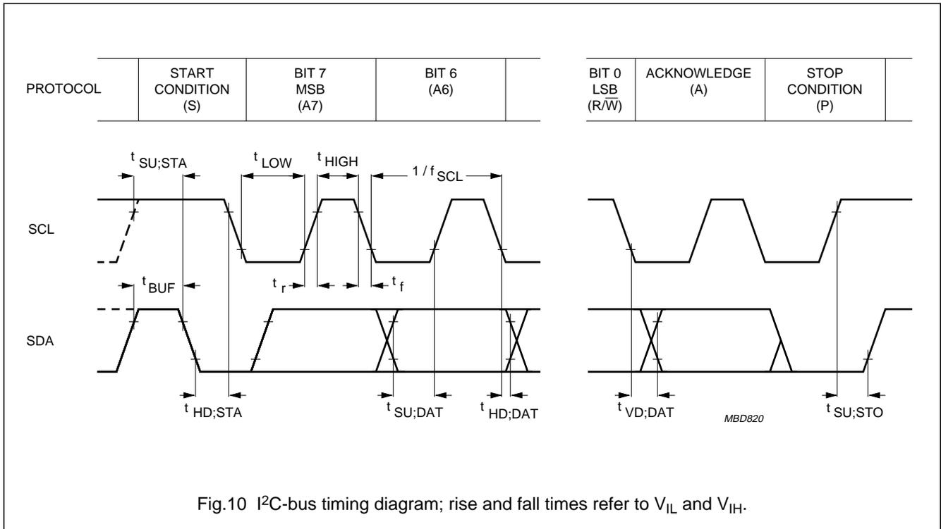
Fig.10 I<sup>2</sup>C-bus timing diagram; rise and fall times refer to V<sub>IL</sub> and V<sub>IH</sub>.
