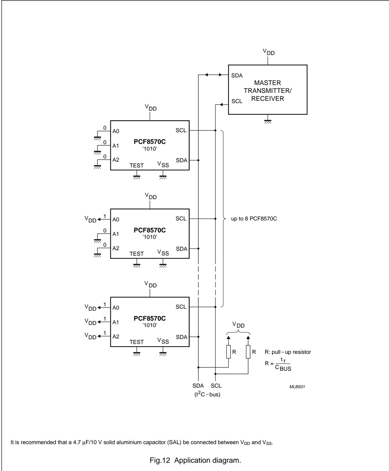
256 × 8-bit static low-voltage RAM with I<sup>2</sup>C-bus interface
