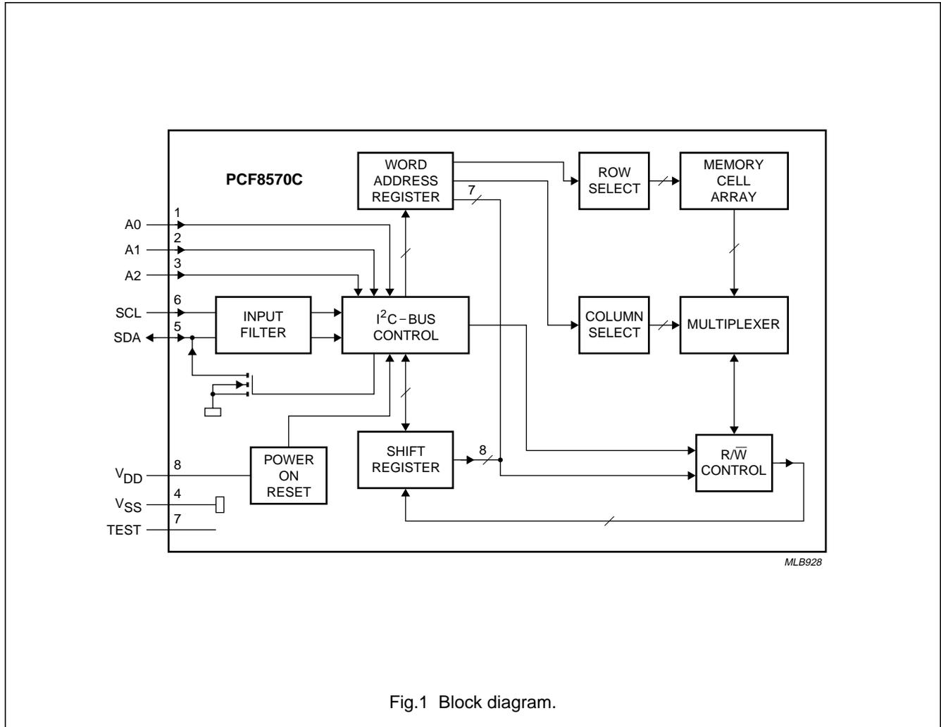
Fig.1 Block diagram.
