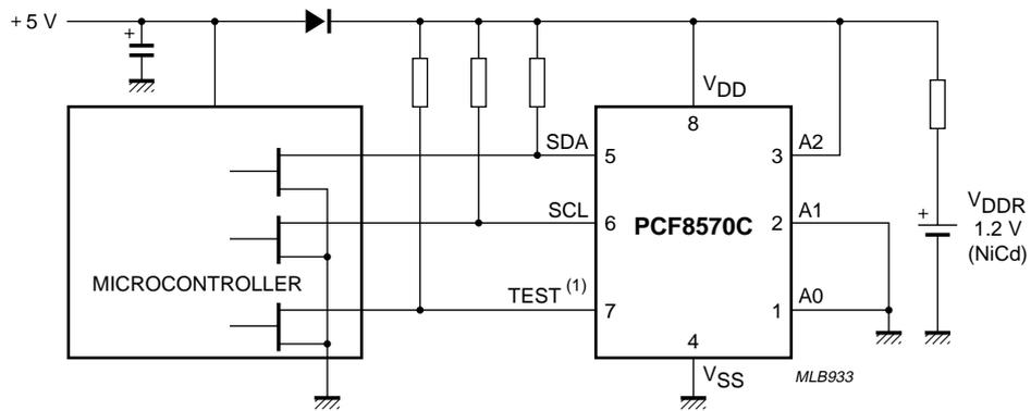
It is recommended that a 4.7 μF/10 V solid aluminium capacitor (SAL) be connected between V<sub>DD</sub> and V<sub>SS</sub>.
