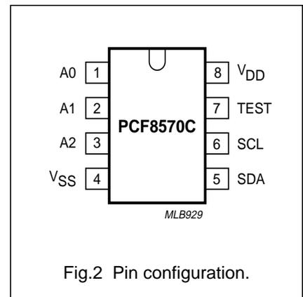
Fig.2 Pin configuration.
