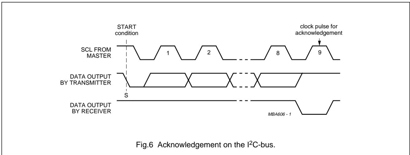
Fig.6 Acknowledgement on the I<sup>2</sup>C-bus.
