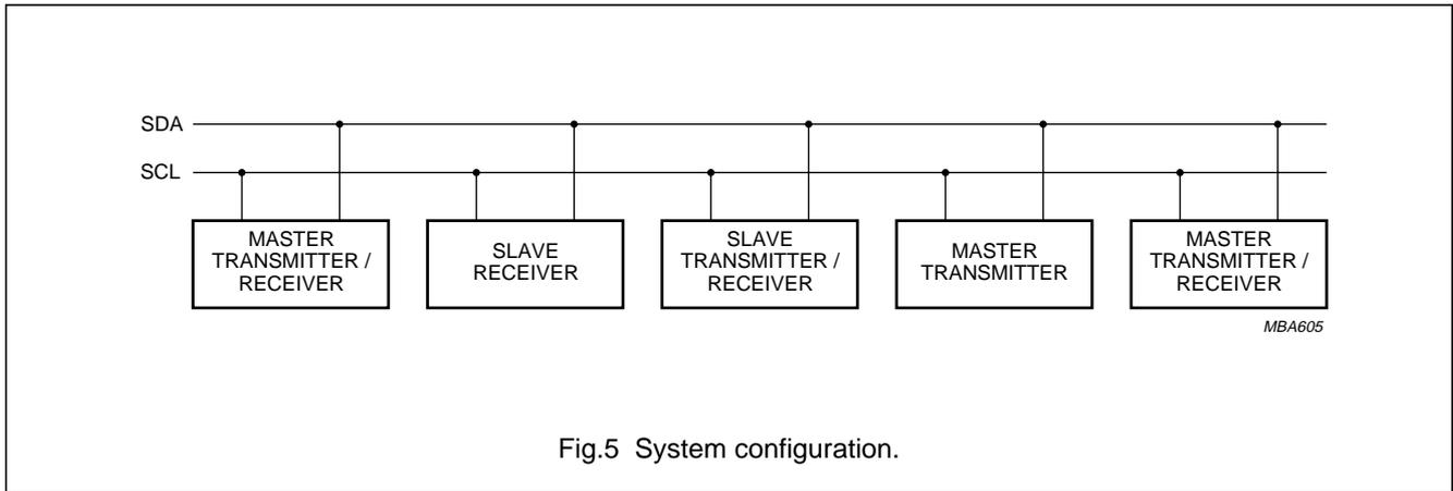
Fig.5 System configuration.
