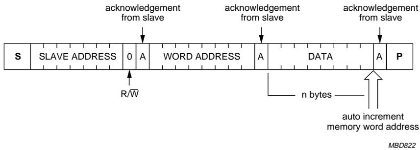
Fig.7 Master transmits to slave receiver (WRITE) mode.
