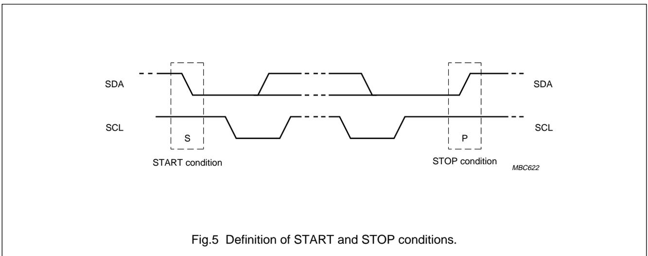
Fig.5 Definition of START and STOP conditions.
