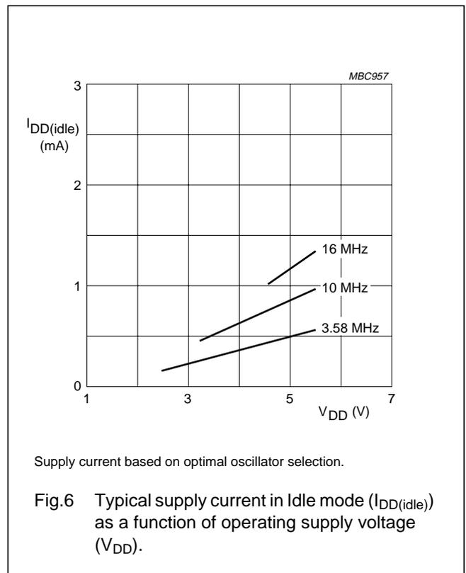
Supply current based on optimal oscillator selection.
