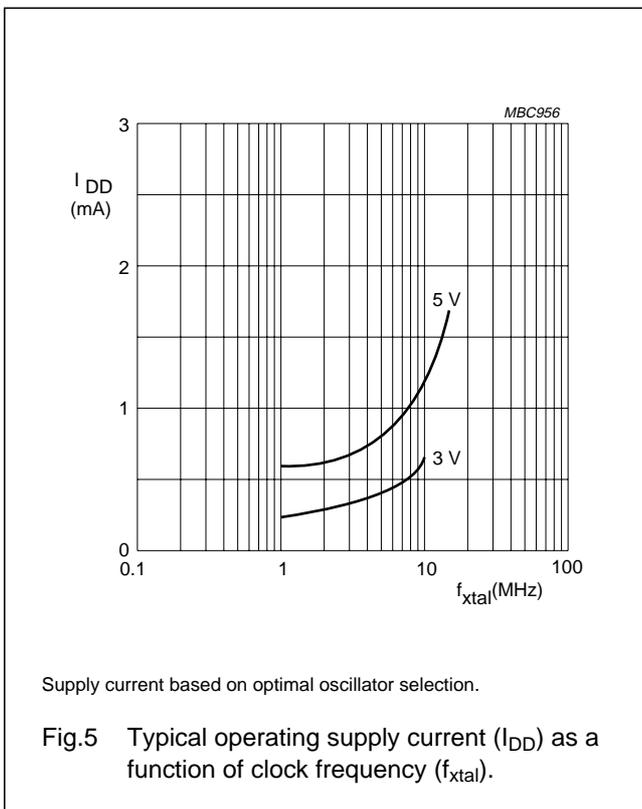
Supply current based on optimal oscillator selection.
