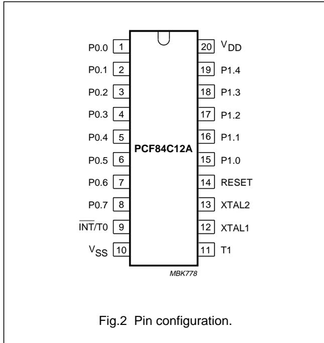
Fig.2 Pin configuration.
