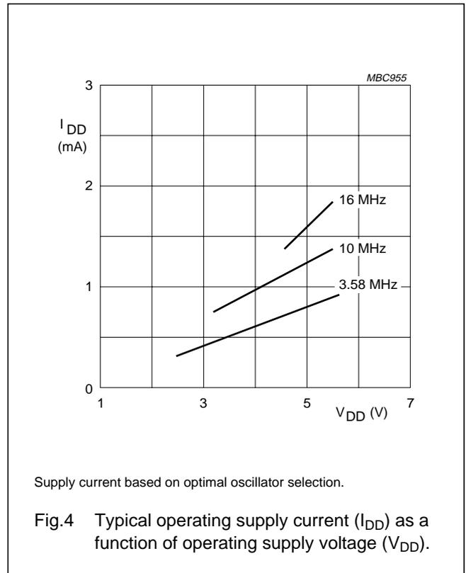
Supply current based on optimal oscillator selection.
