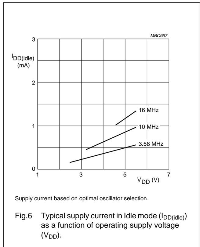
Supply current based on optimal oscillator selection.
