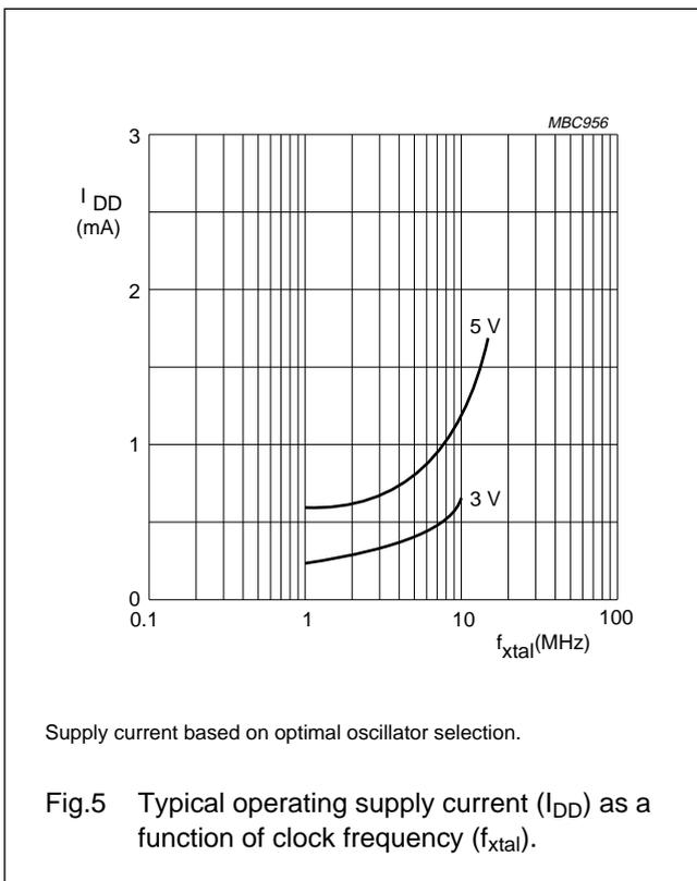
Supply current based on optimal oscillator selection.
