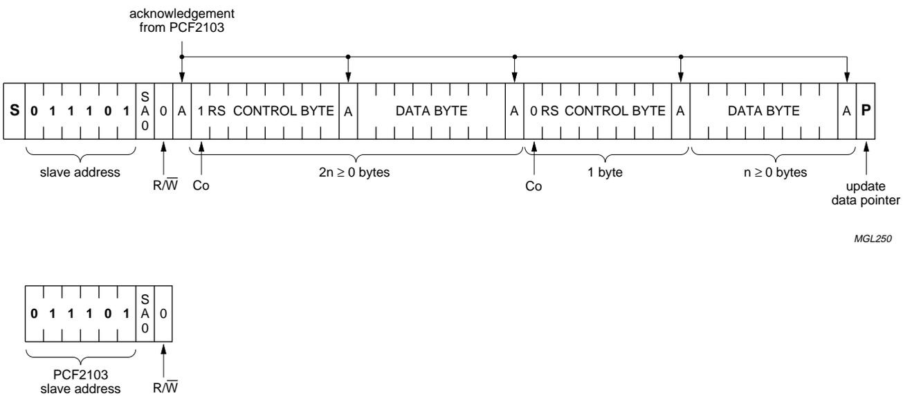
Fig.19 Master transmits to slave receiver; write mode.
