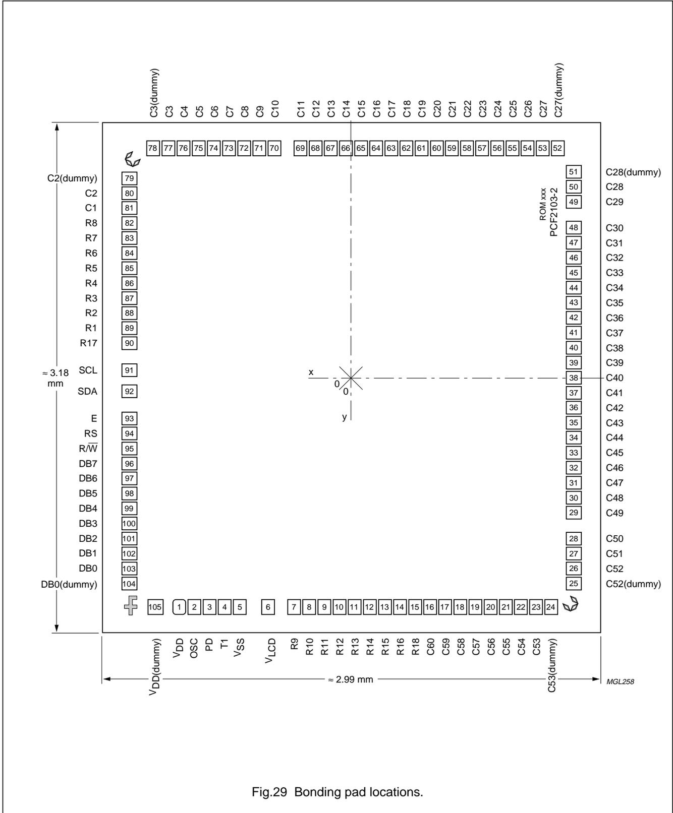
Fig.29 Bonding pad locations.
