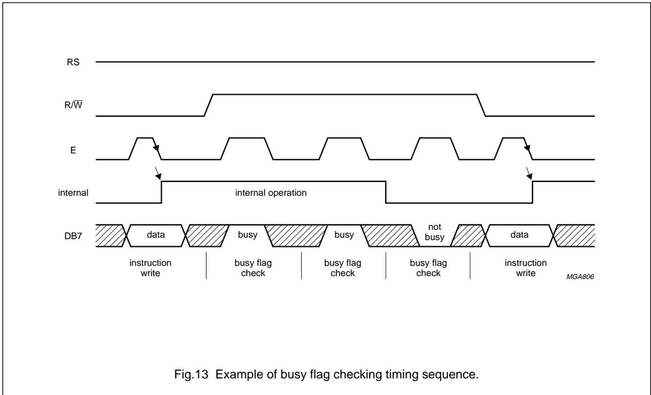
Fig.13 Example of busy flag checking timing sequence.
