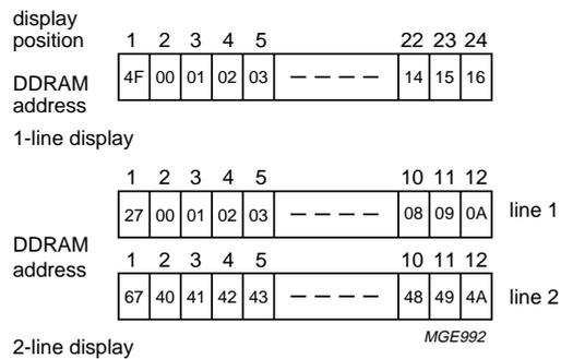
Fig.3 DDRAM-to-display mapping: right shift.
