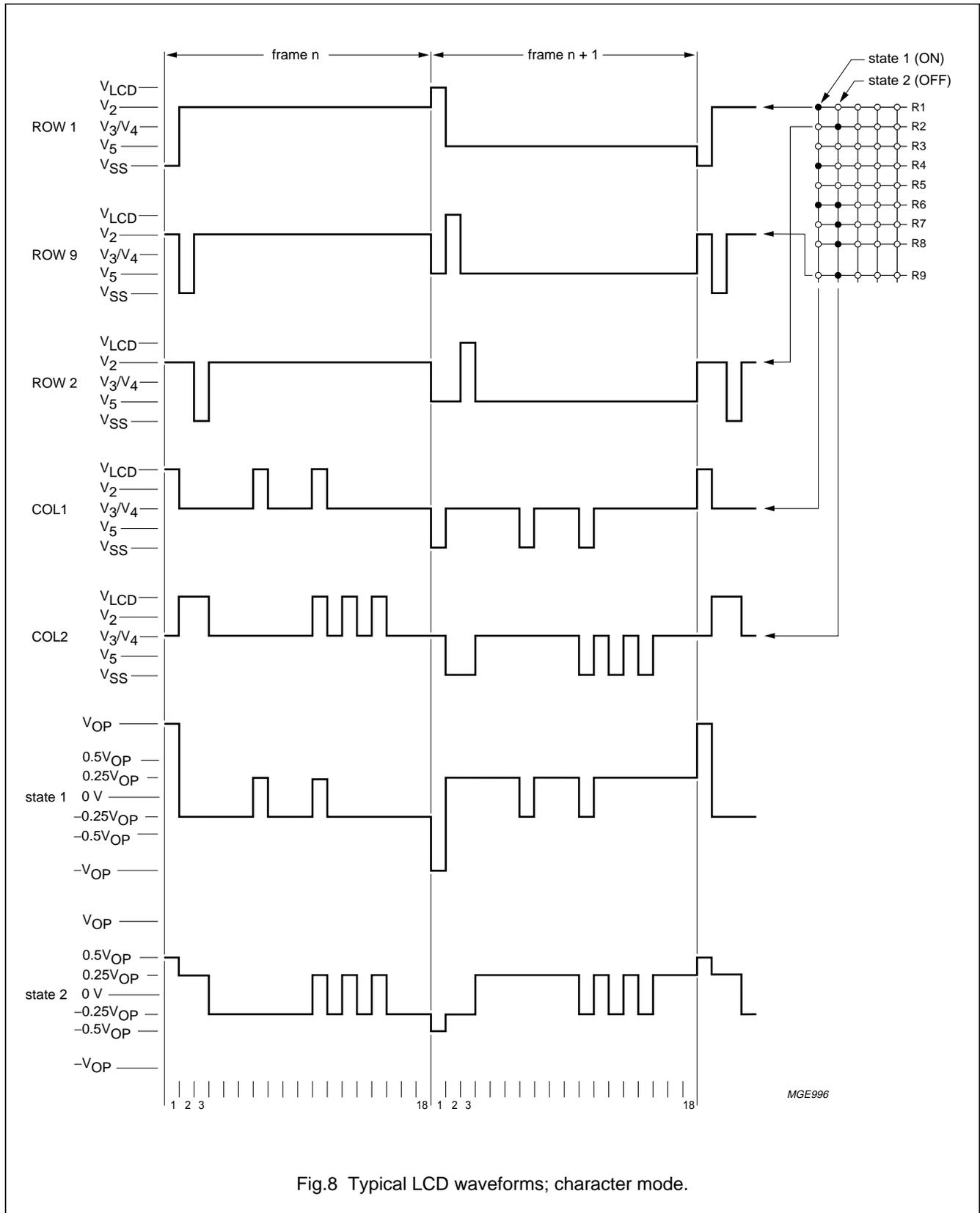
Fig.8 Typical LCD waveforms; character mode.
