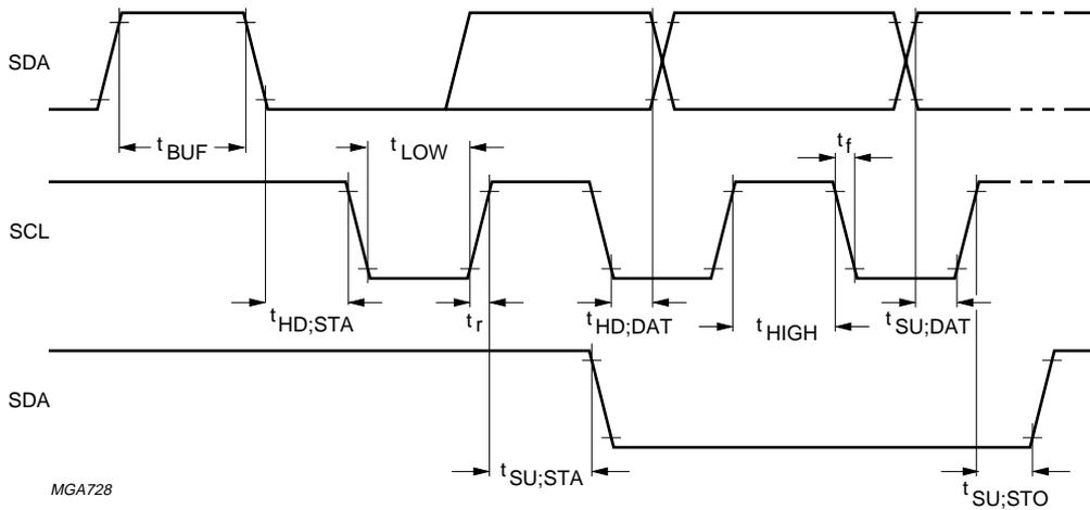
Fig.22 I<sup>2</sup>C-bus timing diagram.
