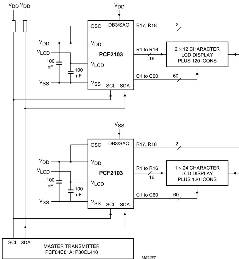
Fig.28 Application using I<sup>2</sup>C-bus interface.
