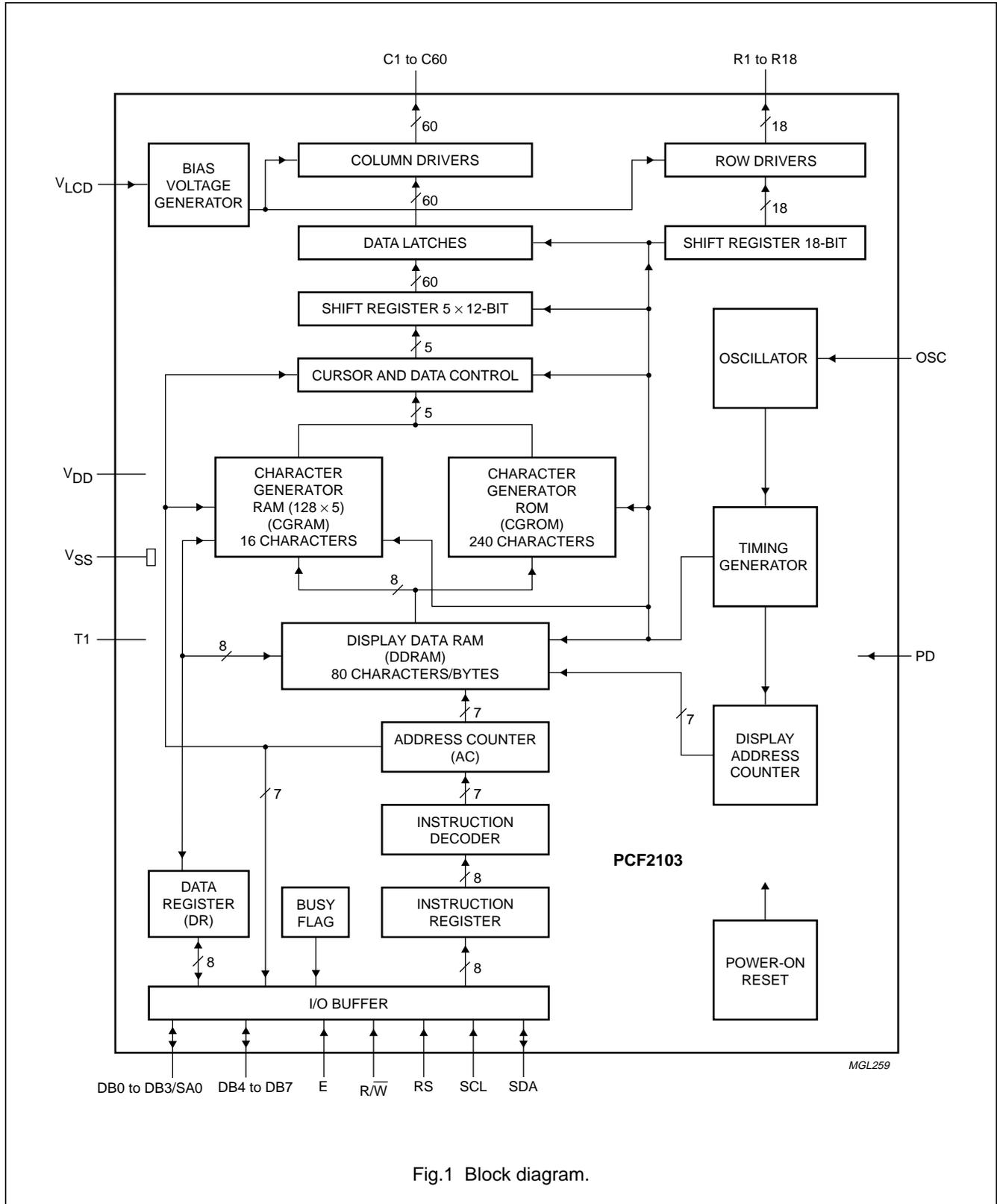
Fig.1 Block diagram.
