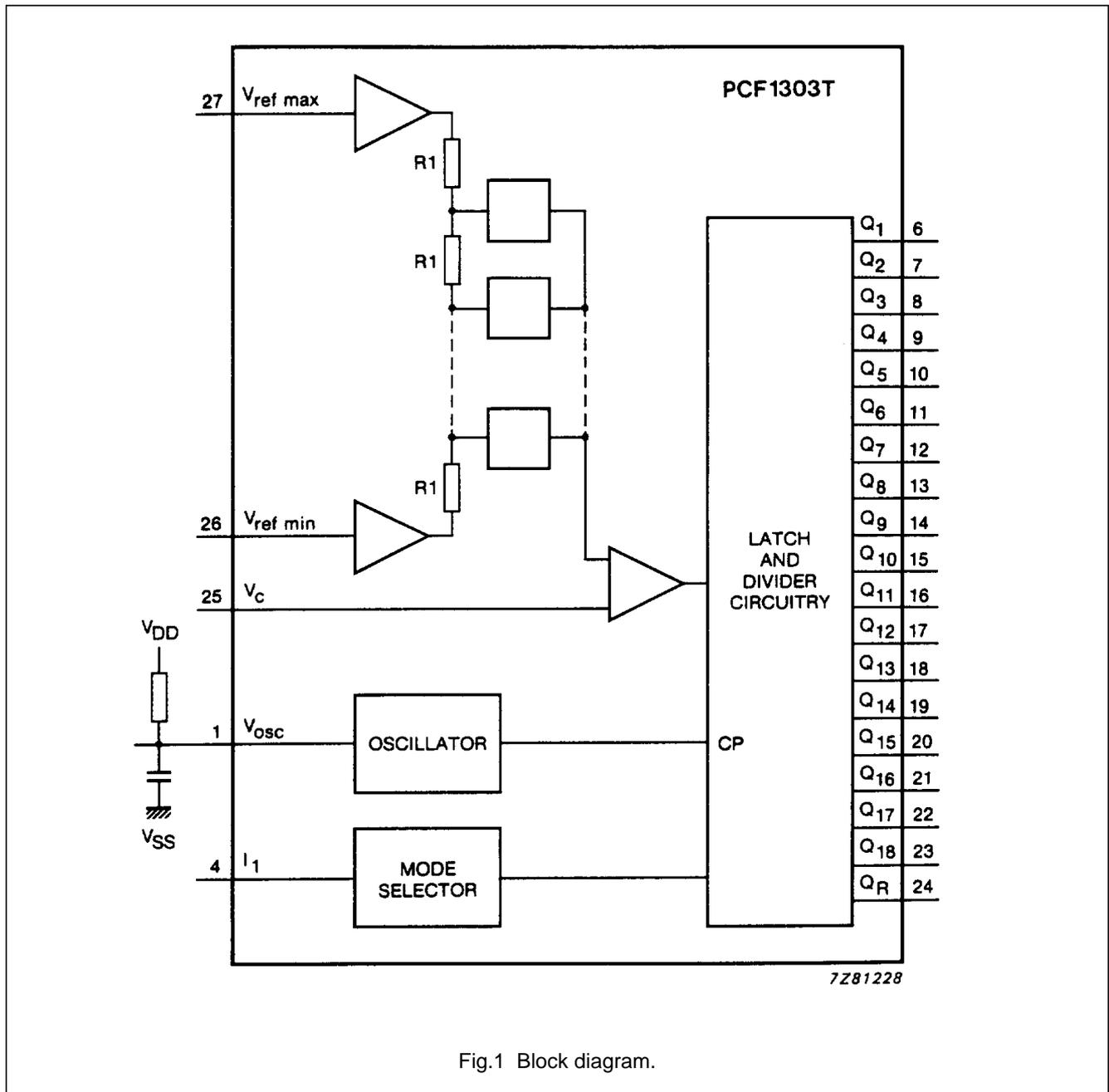
Fig.1 Block diagram.
