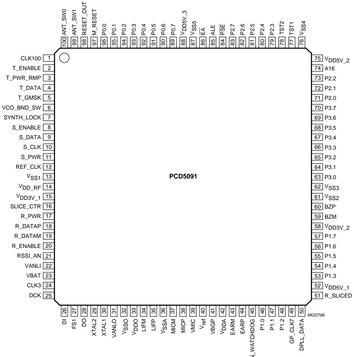
Fig.3 Pin configuration (LQFP100).
