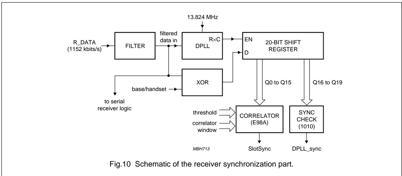
Fig.10 Schematic of the receiver synchronization part.
