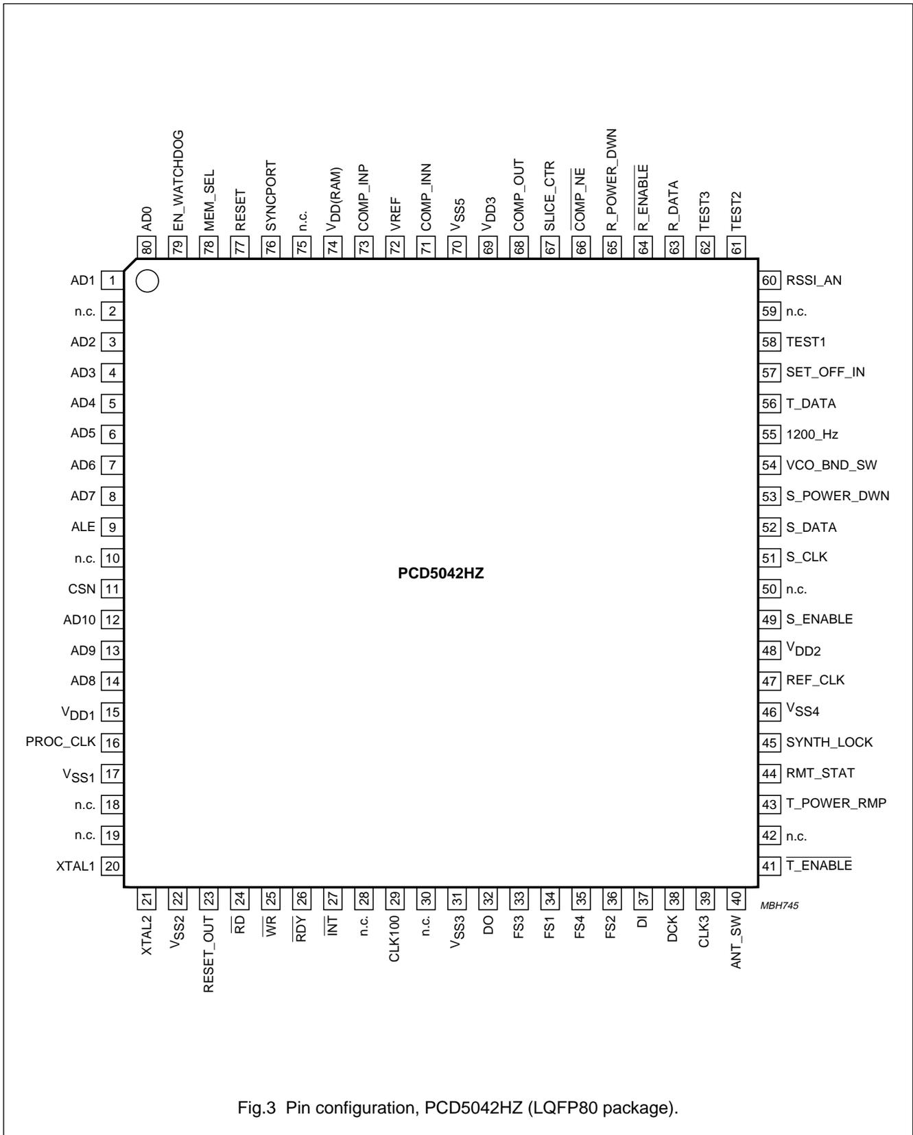
Fig.3 Pin configuration, PCD5042HZ (LQFP80 package).
