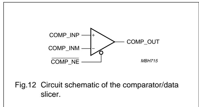
Fig.12 Circuit schematic of the comparator/data slicer.
