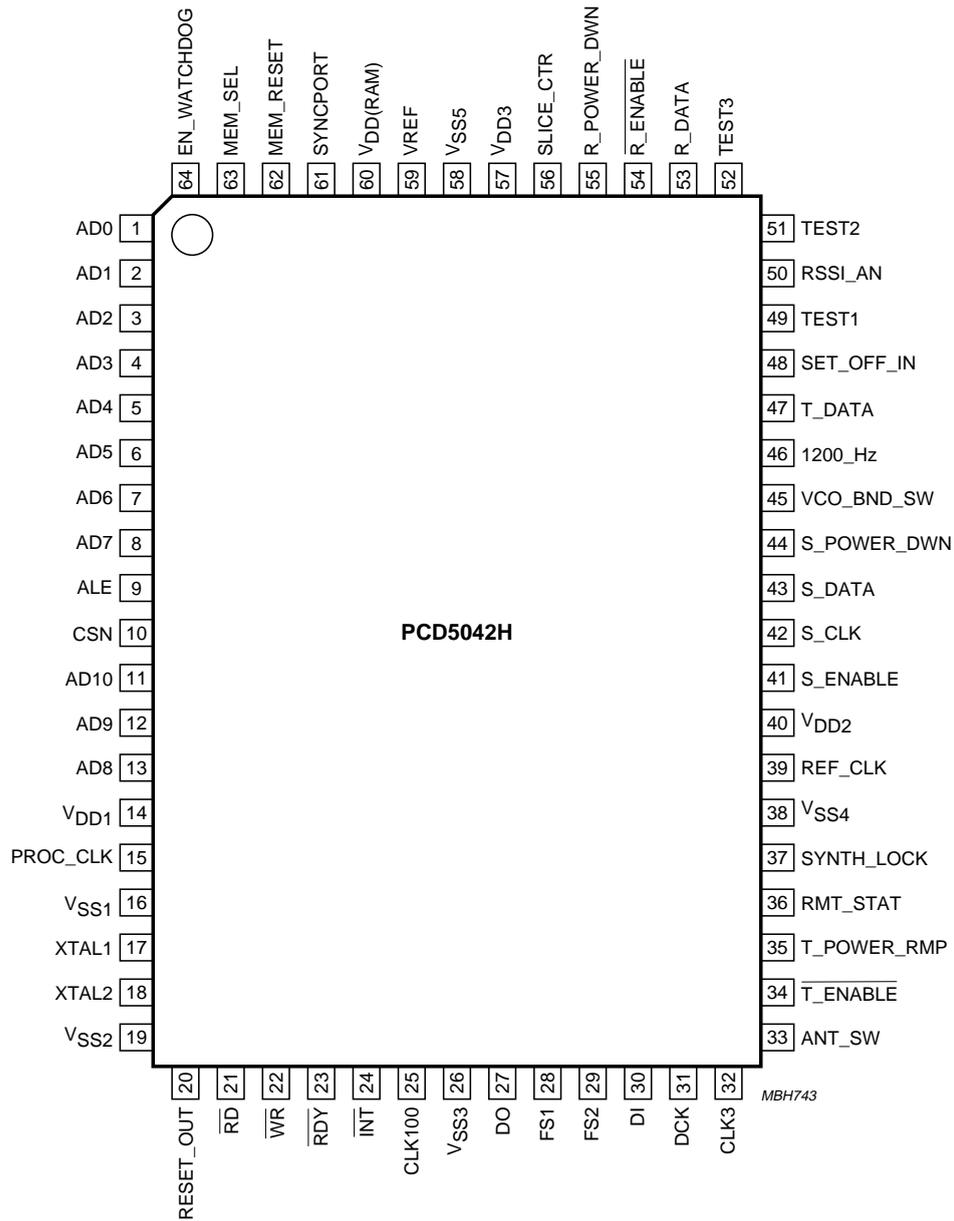
Fig.2 Pin configuration, PCD5042H (QFP64 package).
