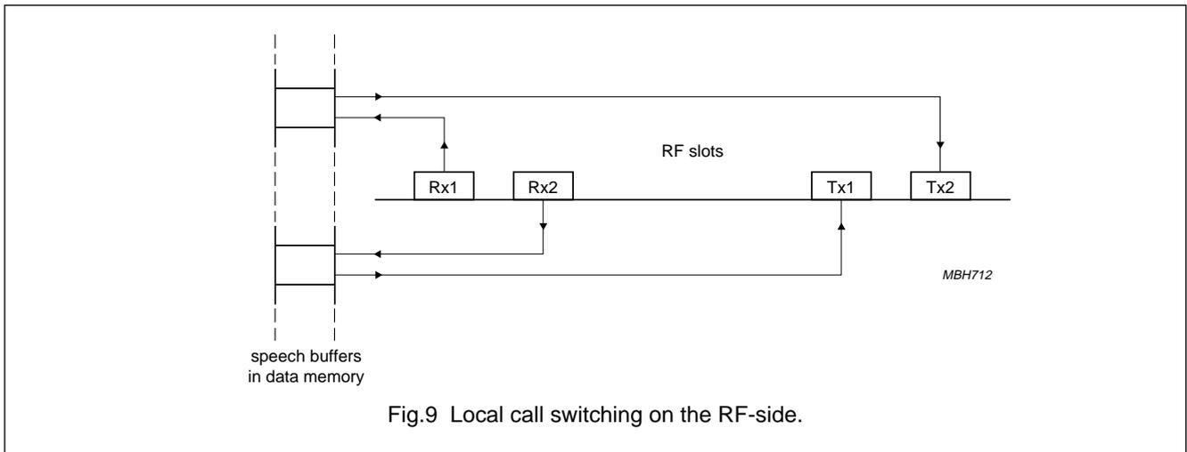
Fig.9 Local call switching on the RF-side.
