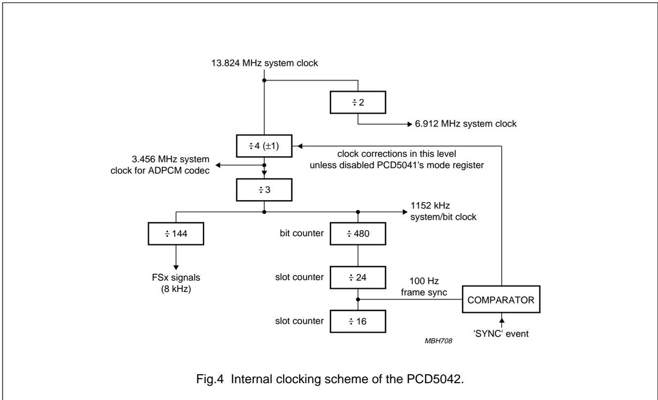
Fig.4 Internal clocking scheme of the PCD5042.
