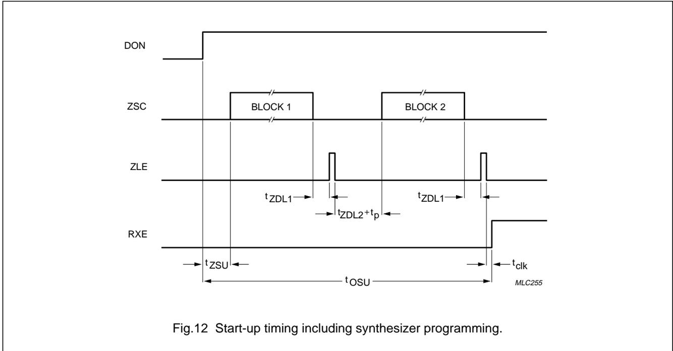
Fig.12 Start-up timing including synthesizer programming.
