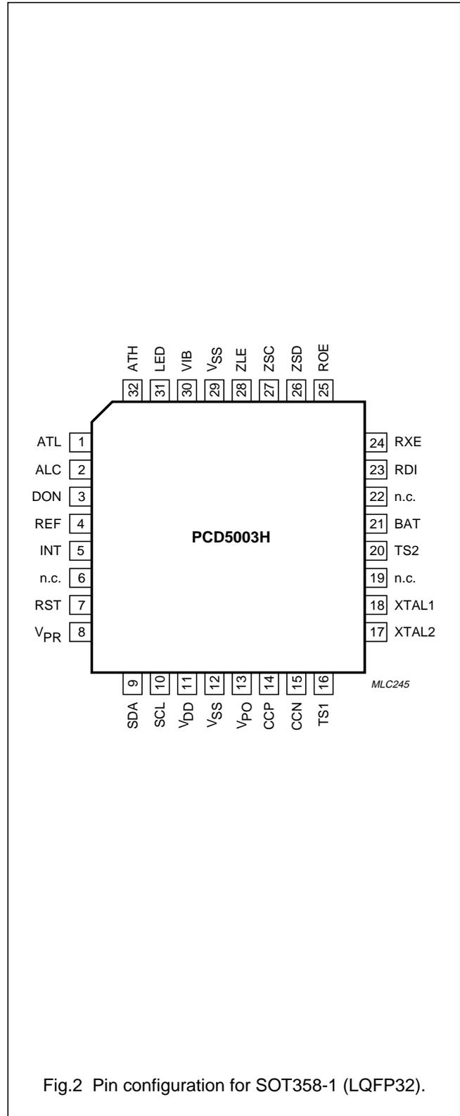
Fig.2 Pin configuration for SOT358-1 (LQFP32).
