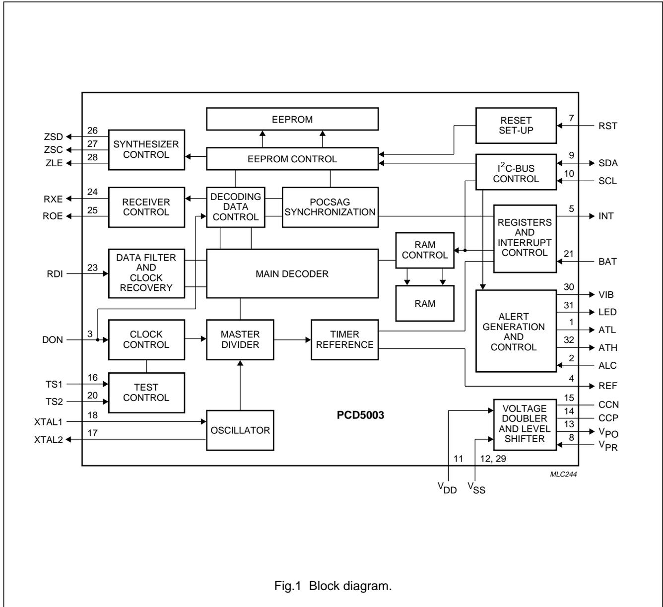
Fig.1 Block diagram.
