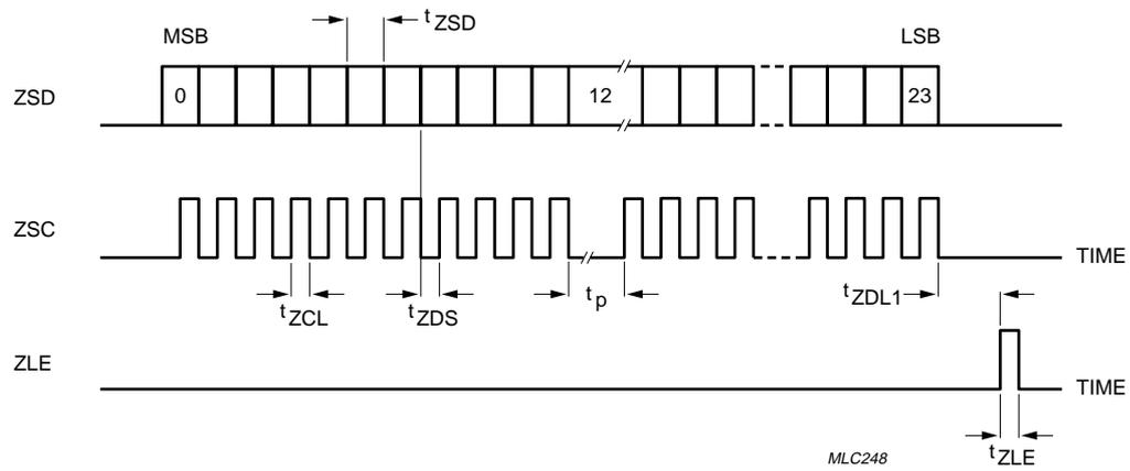
Fig.5 Synthesizer interface timing.
