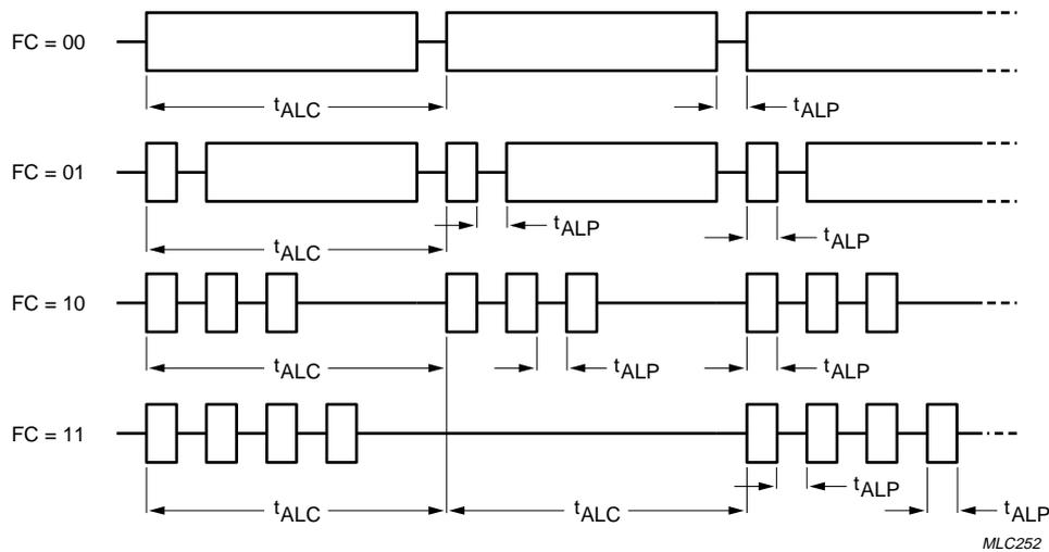
Fig.9 POCSAG alert timing.
